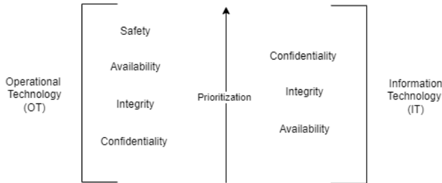
Figure 2.2: General priorities for the security objectives when concerning typical IT systems vs. OT systems. The figure is adopted from [GTA+22].
