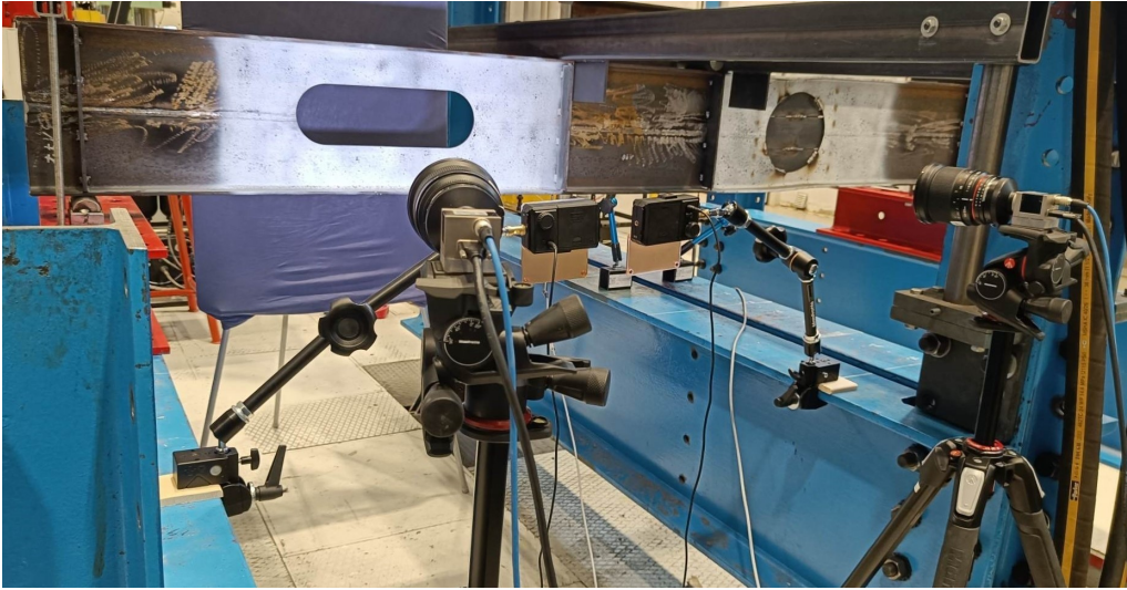
Figure 2.10: Two cameras at distinct angles for 3D DIC depth of view.
