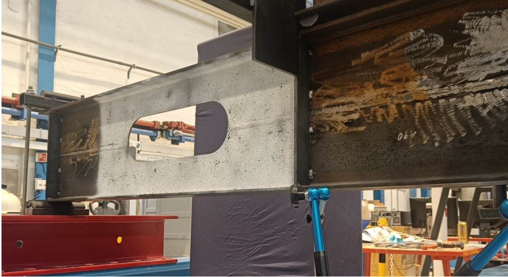
Figure 2.18: The early stages of the bending test of specimen G. No visible deformations were observed.
