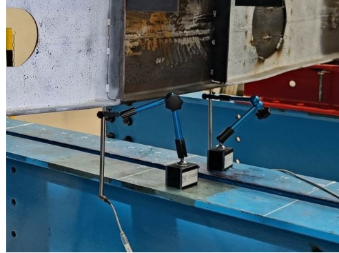
(b) The LVDT placement on specimen G.
