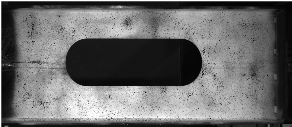
Figure 2.9: Spray-painted opening region for DIC meshing on specimen G.
