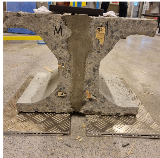
Figure 5.6: Steel plate foundation
