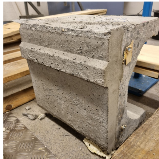
Figure 5.8: Residual joint after separation
