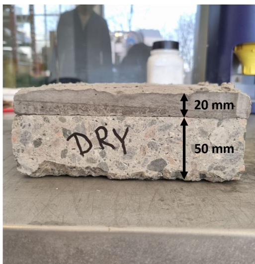
Figure 5.11: Cast HCS sample with measurements
