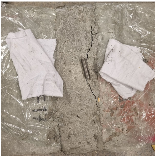
Figure 5.5: Location of steel dowel and rags
