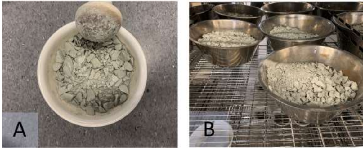
Figure 10. A. Manual grinding of clay to smaller pieces. B. Drying of manually grinded clay in the cabinet at 105°C for 36 more hours.
