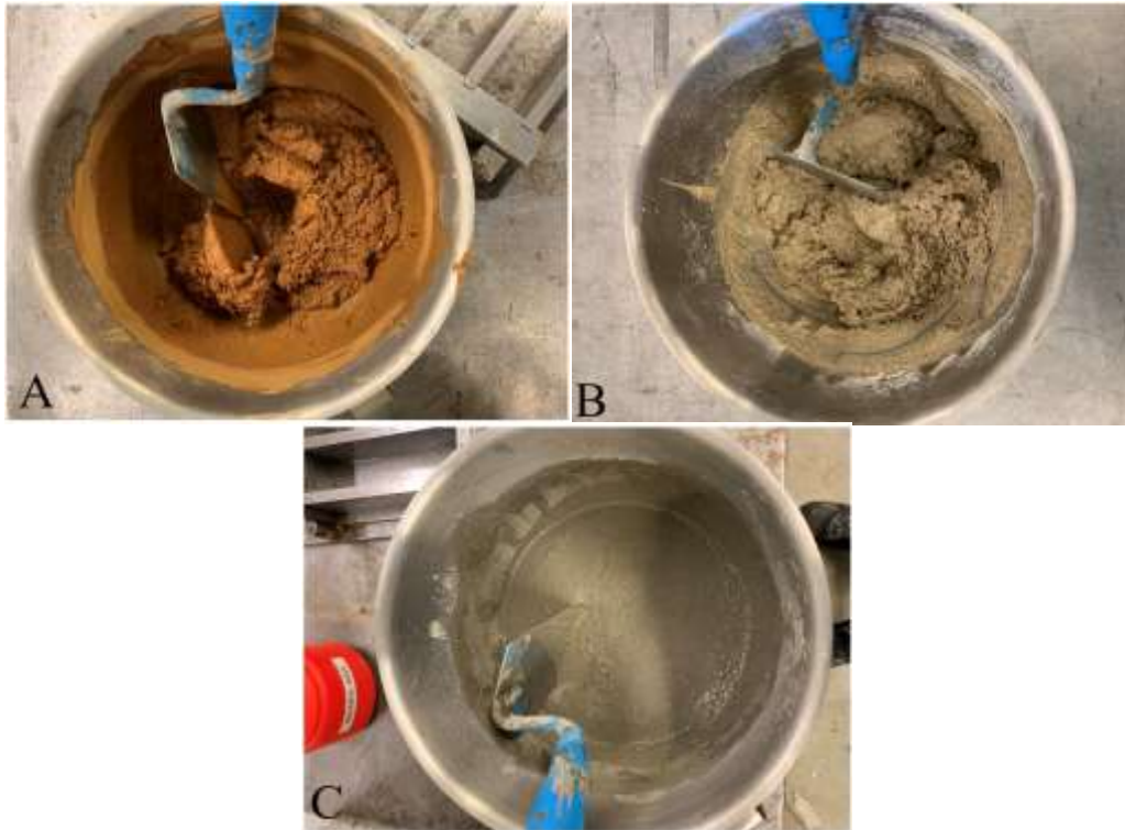
Figure 16. Shows the mixing of the materials. A. Local marine clay, B. Pottery white clay and C. standard cement (reference).
