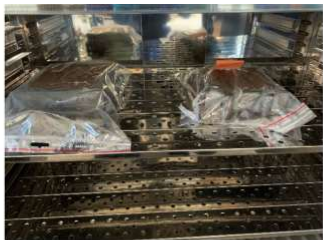
Figure 18. shows curing of samples in the heating cabinet at 60^\circ\text{C} for (22 \pm 2) hours.
