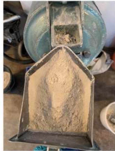
Figure 11. Shows the grinding process of the clay with the grinder from SINTEF.
