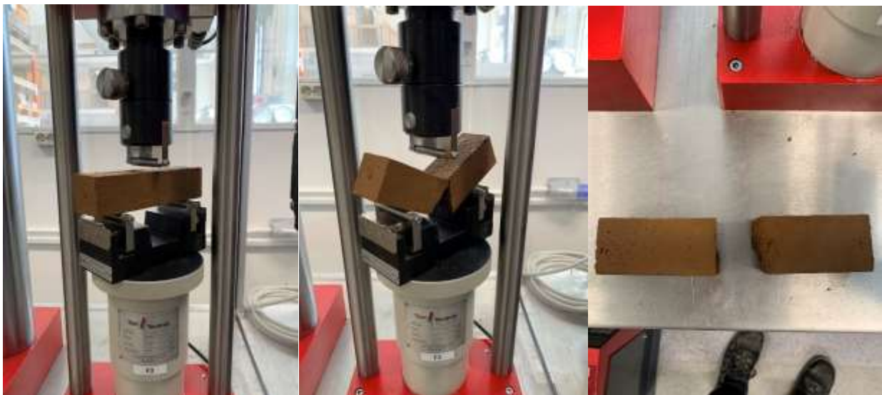
Figure 39. Local marine clay specimen during the flexural test
