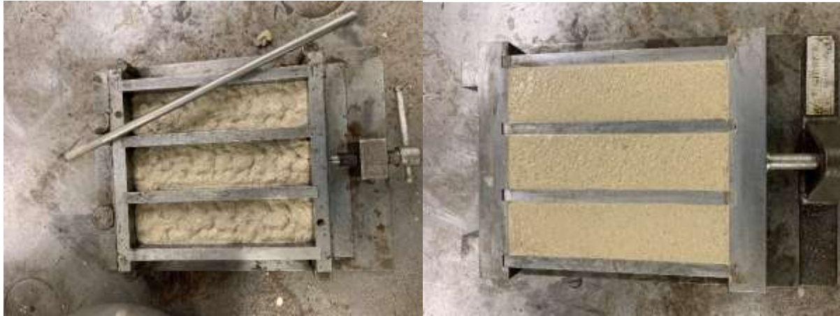
Figure 17. Casting process: The moulds were filled halfway, compacted with trowel and shovel, then the moulds were completely filled with mortar and the compacting procedure was repeated. A vibrating table was used during casting.
