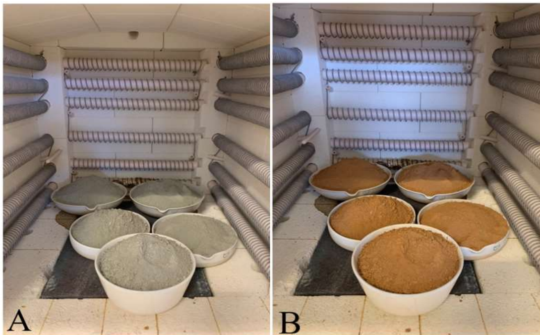
Figure 13. Calcination process of local marine clay at 600°C, 700°C, and 850°C. A. shows the clay in the oven before calcination and B. shows the clay after the calcination.
