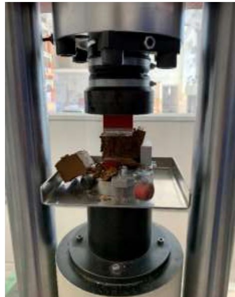
Figure 22. Shows the compressive strength test of local marine clay.
