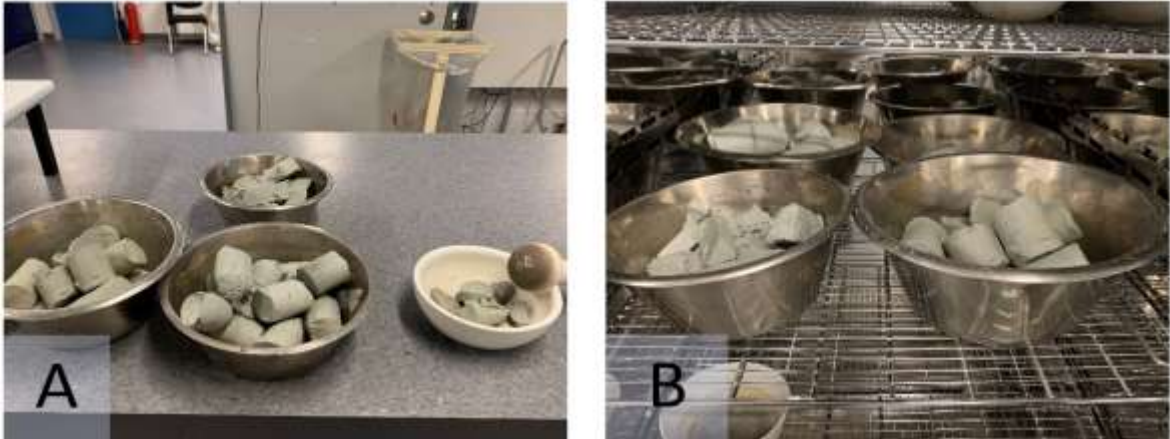
Figure 9. A. shows the local marine clay sliced into pieces and B. shows the clay materials were dried in the drying cabinet at 105°C for 36 hours.
