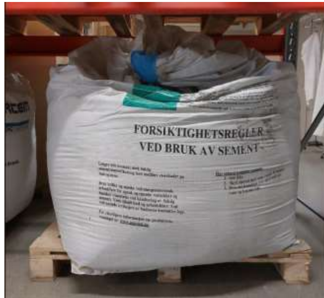
Figure 5. The standard cement FA (CME II) form Norcem used in this project.
