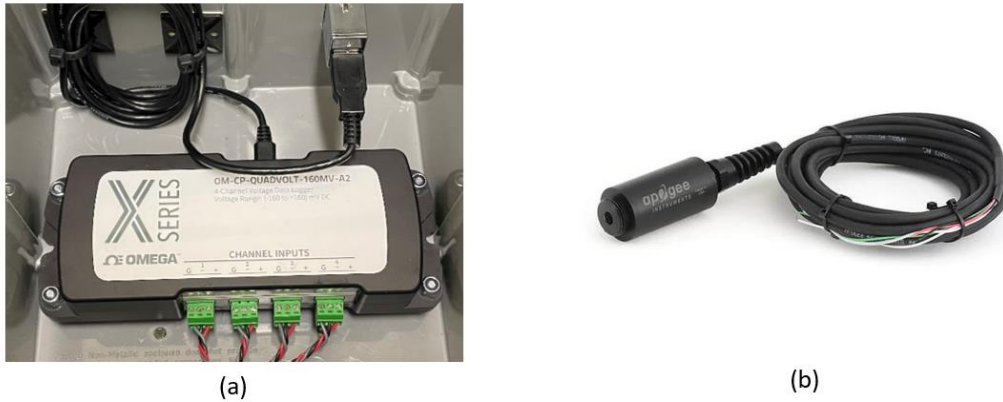
Figure 2.8: (a) An example of a data logger that can be used for the OCT. The photo is taken at UlaVal by Dr. Jan Lindgård. (b) Oxygen sensor (Apogee SO-200 Series), picture taken from [58].
