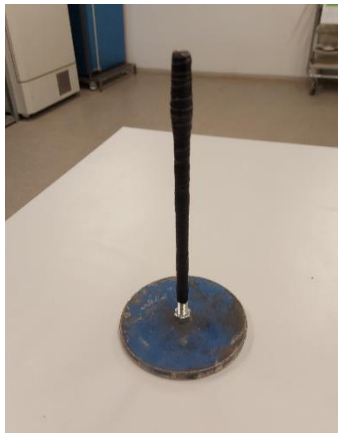
Figure 3: The steel pestle used for compacting the aggregate material prior to OCT testing.
