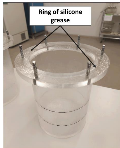
Figure 8: The picture shows how silicon grease should be applied on the top surface of the reaction cell.
