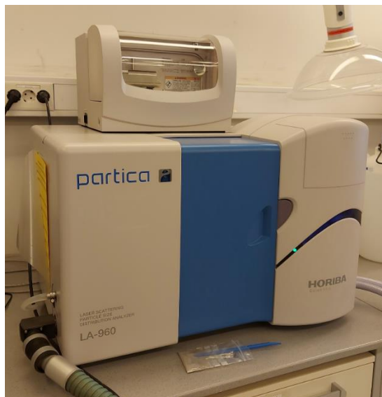
Figure 6.12: The picture shows Horiba LA-960 (otherwise known as the Laser Scattering Particle Size Distribution Analyzer ).
