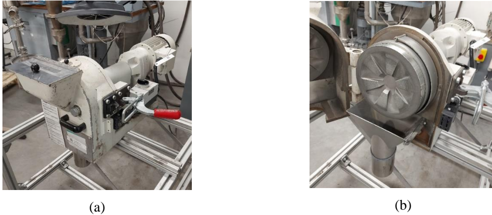
Figure 6.2: The figure shows the FRITSCH Disk Mill PULVERISETTE 13 . Picture (a) shows how the machine looks from the outside and picture (b) shows the disks (steel disks are shown in the picture, but tungsten disks were used in sample preparation for this thesis).
