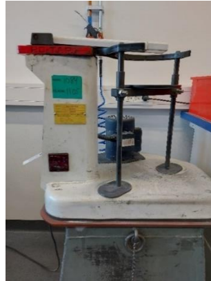
Figure 6.9: The picture shows the RO-TAP RX-29 Sieve Shakers .
