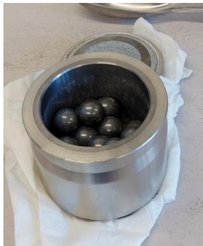
Figure 6.7: The figure shows the grinding set (tungsten-lined bowl and tungsten balls) of the planetary mill.
