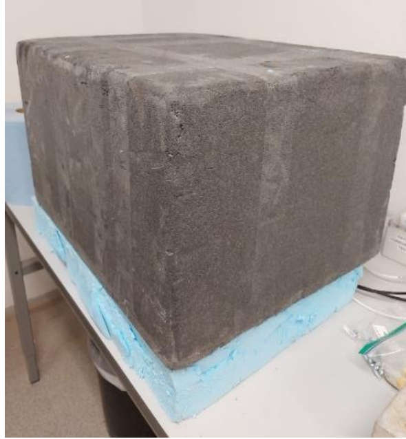
Figure 6.16: The picture shows the polystyrene case used to keep the reaction cell in an environment of constant temperature.
