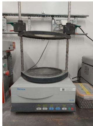
Figure 6.10: The picture shows the RETSCH AS 300 Vibratory Sieve Shaker .
