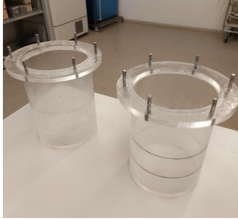
Figure 1: The two reaction cells used for the OCT testing at SINTEF.
