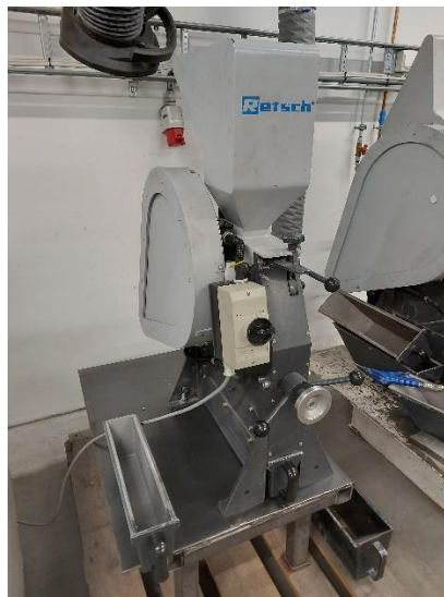
Figure 6.1: The figure shows the RETSCH BB100 jaw crusher used for sample preparation.
