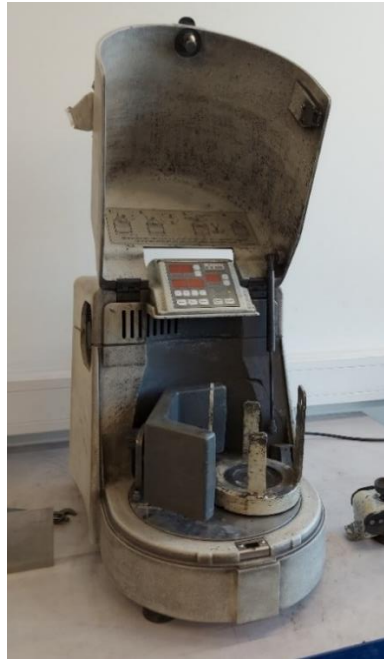
Figure 6.6: The figure shows the planetary mill FRITSCH Planetary Mono Mill PULVERISETTE 6 .
