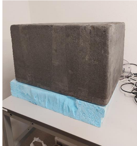
Figure 4: The polystyrene case (and its blue base) used to thermally insulate the reaction cells during the OCT.
