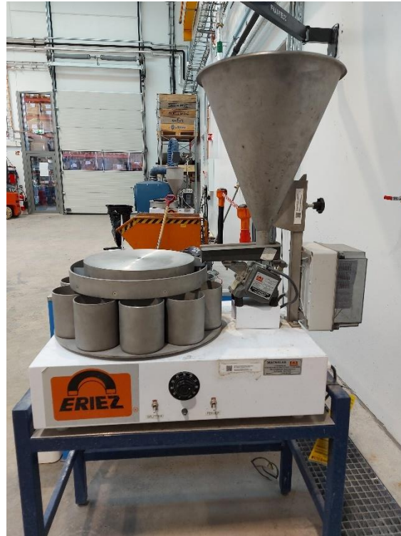
Figure 6.11: The figure shows the 10-chamber MACSALAB Cascade rotary splitter .
