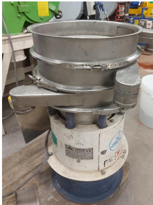
Figure 6.8: The figure shows the SWECO Separator with a sieve tower consisting of the 142 \mu\text{m} and 77 \mu\text{m} sieves. During sample preparation, these sieves (all 42.2 cm in diameter) with the following openings were exclusively used with the SWECO Separator : 77 \mu\text{m} , 142 \mu\text{m} , 4 mm and 20 mm.
