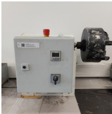
Figure 6.3: The figure shows the bench ball mill used for further grinding of OCT samples.
