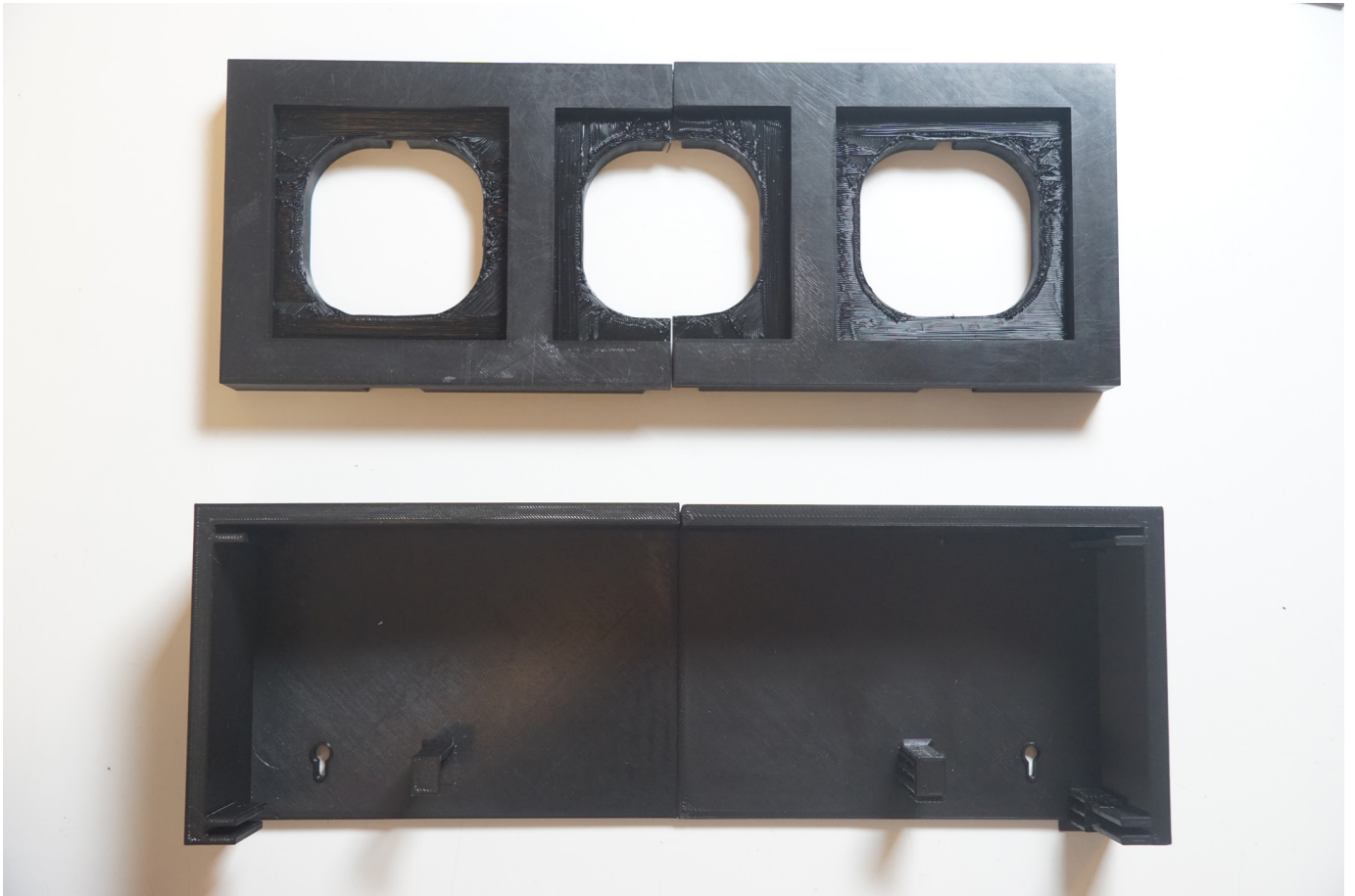
Figure 48. Full scale protoype of front and back panel
