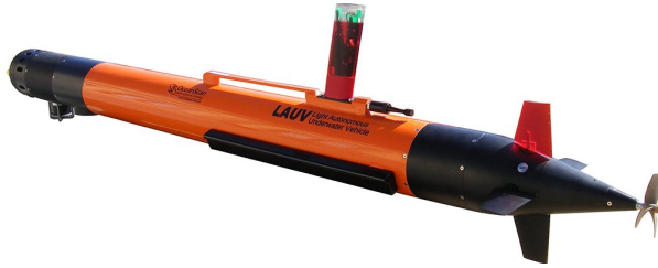
Figure 10.1: The LAUV modeled in this simulation study. Image is taken from OceanScan website (OceanScan - MST; 2023).
