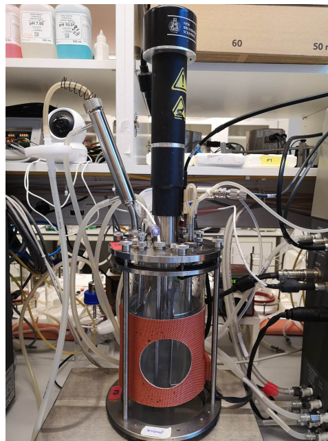
Figure 2.2: A picture of the type of bioreactor that was used in this work.
