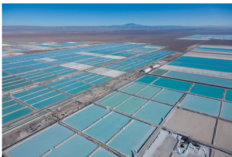
Figure 2: Left: Pools of lithium-enriched water drying in the sun. Right: Lithium carbonate salt after the drying process has been completed. Taken from: (Barranco, 2022; New Technique Could Reduce Lithium-from-Brine Extraction Time to Just Hours.)
