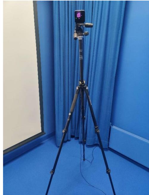
Figure 8: HTC Vive Base station for tracking
