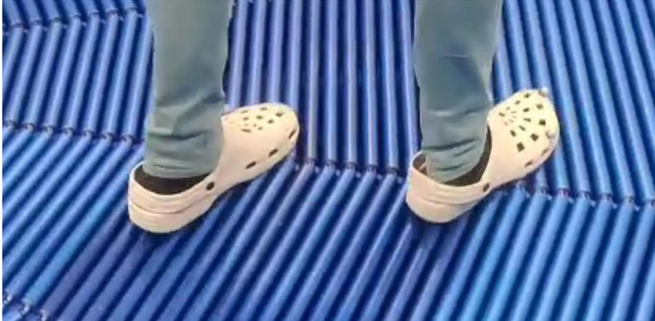
*Figure 26: Feet sideways on the Omnideck while turning*
