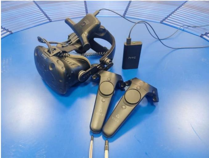
Figure 9: HTC Vive HMD, Wireless adapter, Controllers, and battery pack
