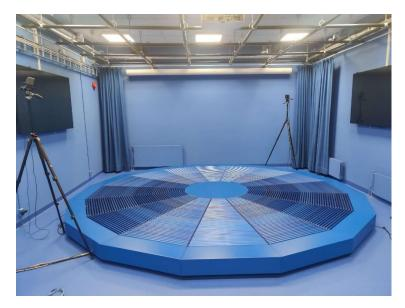
Figure 1: The Omnideck at the Visualization Lab at NTNU
