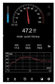
*Figure 33: Sound level meter indicating 47.2 dB*
