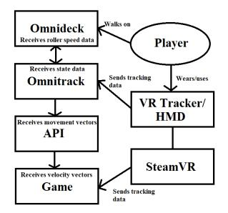
Figure 3: Flow of data between the used technologies
