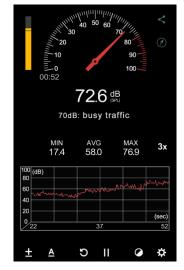
Figure 32: Sound level meter indicating 72.6 dB
