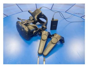
*Figure 9: HTC Vive HMD, Wireless adapter, Controllers, and battery pack*
