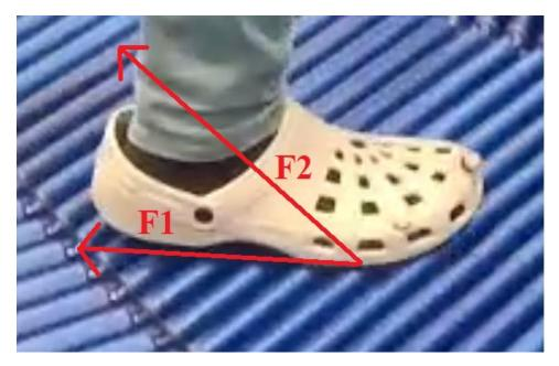
Figure 25: Foot on an exaggerated angle, The F1 vector shows the foot's natural backward movement, The F2 vector shows the Omnideck segment's force vector
