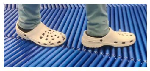
Figure 22: Foot between rollers
