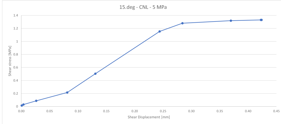
Figure 3.26: Shear stress-displacement for CNL to last converged increment
