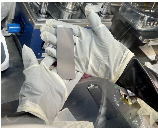
Figure 32: Cathode material (Lithium Cobalt Oxide, LCO) from the Melasta cell with Aluminum (Al) current collector.
