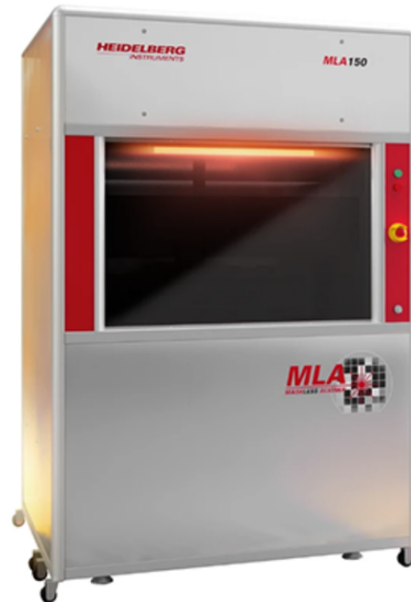
Figure 3.4: The Maskless Aligner MLA150 facilitates the photolithography procedure where photoresist is exposed to UV light in order to become soluble [59]
