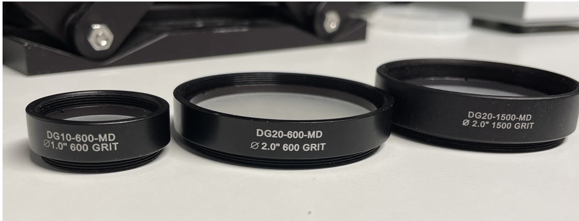
Figure 4.4: Showcase of the three THORLAB diffusers, DØ10-600-MD, DG20-600-MD and DØ20-1500-MD, which are responsible for providing homogenous light distribution of better visualisation of the droplet and the particles within.
