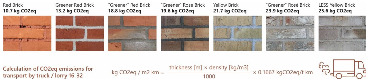
Figure 4.3: Bricks from the Unboxing Carbon Catalog used to analyse the effect of including the transport distance (A4) to the emissions per square meter.
