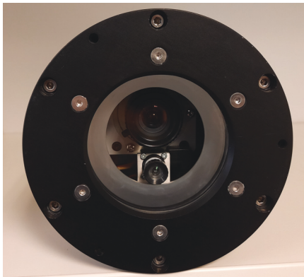
(a) Front-view of the UHI-4 by Ecotone. The large lens is the HSI, while the smaller lens is an RGB imager.
