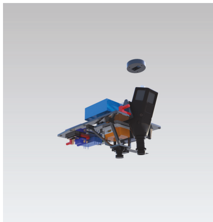
(b) CAD illustration of a micro-payload developed by Oliver Hasler and it integrates an HSI-v4 (160 grams), a downwelling irradiance spectrometer, an IMU, an RGB camera and processing units. Total payload weight is 500 grams. Courtesy of Oliver Hasler.
