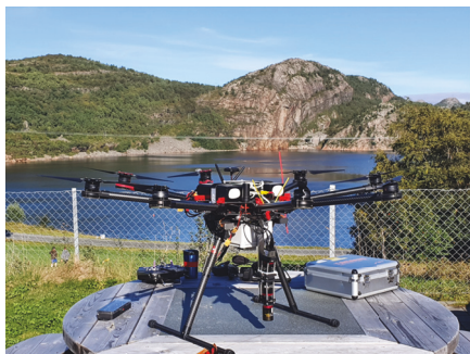
(c) The UAV is a DJI S1000 equipped with an HSI-v6. Courtesy of Pål Kvaløy.
