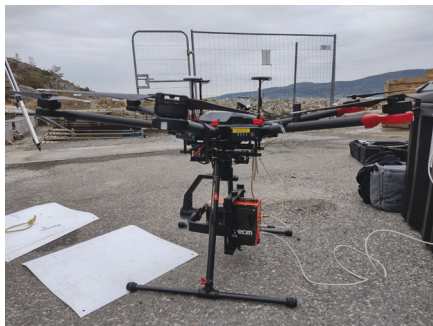
(a) DJI M600 with a Specim AFX10 on a gimbal. Courtesy of Joseph Garrett.
