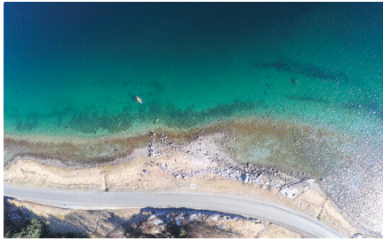
(a) Zoom-in of a GoPro image from a UAV, from the experiment in [36]. Flickering sunflint is seen, caustics on the seafloor, and generally reduced visibility towards deeper water.
