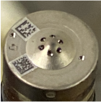
(a) Not welded injector.
