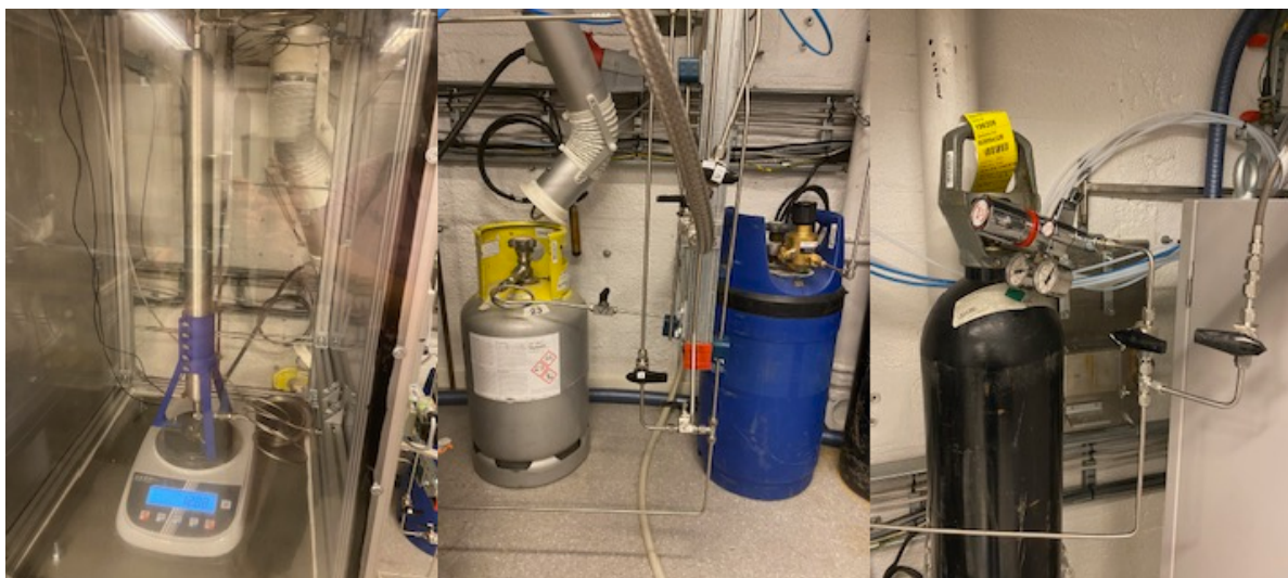
Figure 48: Pictures of the cylindrical fuel tank on the weight (to the left), the ammonia supply tank (grey in the centre) and the nitrogen supply tanks (blue and black, to the right).
