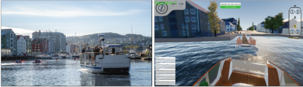
Figure 1: Left: Autonomous urban passenger ferry milliAmpere2 during public trial operations. Right: Simulation of remote supervisory control of milliAmpere2 at NTNU Shore Control Lab
