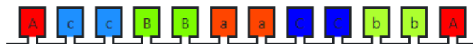
Fig. 12. Illustration of 36s6p winding layout. Represented with a third of the full configuration [33].
