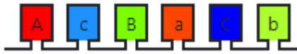
Fig. 13. Illustration of the winding layout for s30p10, s18p6 and s24p8. The figure represents a fifth of the s30p10 configuration, a third of the s18p6 configuration, and a fourth of the s24p8 configuration [33].
