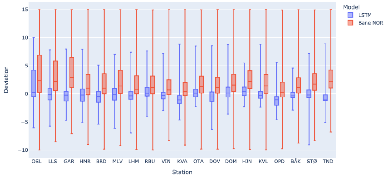
Figure 6.3.3: Box plot showing the distribution of the quantitative values of estimate deviation for both models, plotted for each station. Estimation deviation boundaries is here set to 10 minutes before and 15 minutes after.
