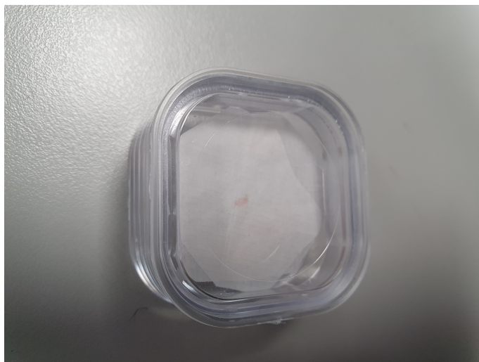
Figure 30: Image of the sample box used for transferring the sample from the FIB to the TEM. It is a membrane box with the sample having been placed between two pieces of cigarette paper.
