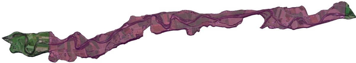
Figure 12: Area of interest inside the 2D flow area from the hydraulic model in HEC-RAS, with the border of the land photo defining the extent of the 2D flow area.
