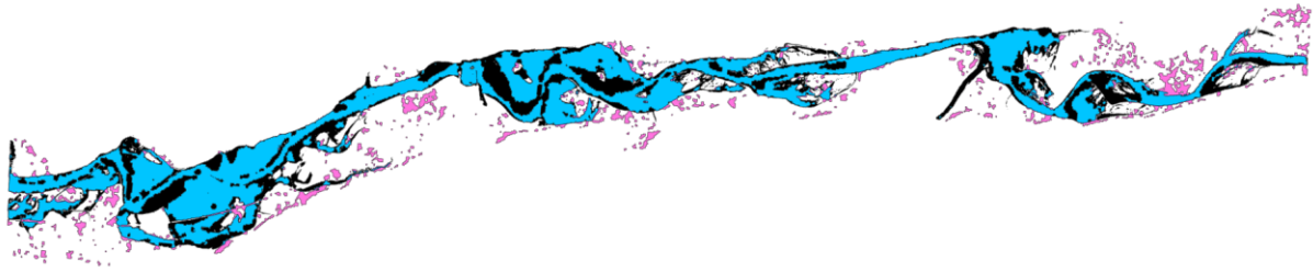
Figure 60: Flood overlay plot from the flood event on November 24, 2021, using best measure of fit Manning's n-values 0.02 in the main channel and floodplains. The blue area indicates the region the simulation and flood delineation map of the SAR image overlap and coincide. The black area represents the over-prediction from the simulation, while the pink is illustrating the under-prediction.
