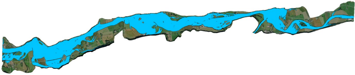
Figure 49: Flood inundation area from the flood event on August 14, 2003, using Manning’s n-values in the main channel from the regionalized calibration.
