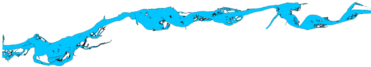
Figure 54: Flood inundation area from the flood event on August 14, 2003, using Manning's n-values 0.1 and 0.2 for the forest, and 0.1 for floodplains. The blue area indicates the region where both simulations overlap and coincide. The black area represents the additional flooded area when a Manning's n-value of 0.2 for forest is used, extending beyond the overlapping region.
