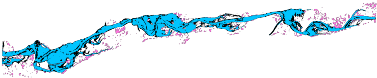
Figure 63: Flood overlay plot from the flood event on November 24, 2021, using best measure of fit Manning's n-values 0.02 in the main channel and floodplains. The blue area indicates the region the simulation and flood delineation map of the SAR image merged with SR16 map overlap and coincide. The black area represents the over-prediction from the simulation, while the pink is illustrating the under-prediction.
