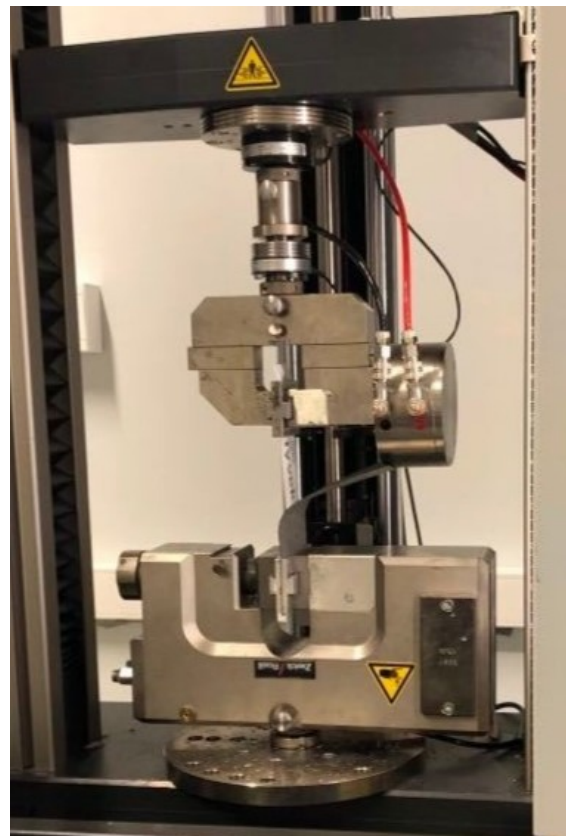
Figure 3.14: Peel resistance specimen in the testing machine.
