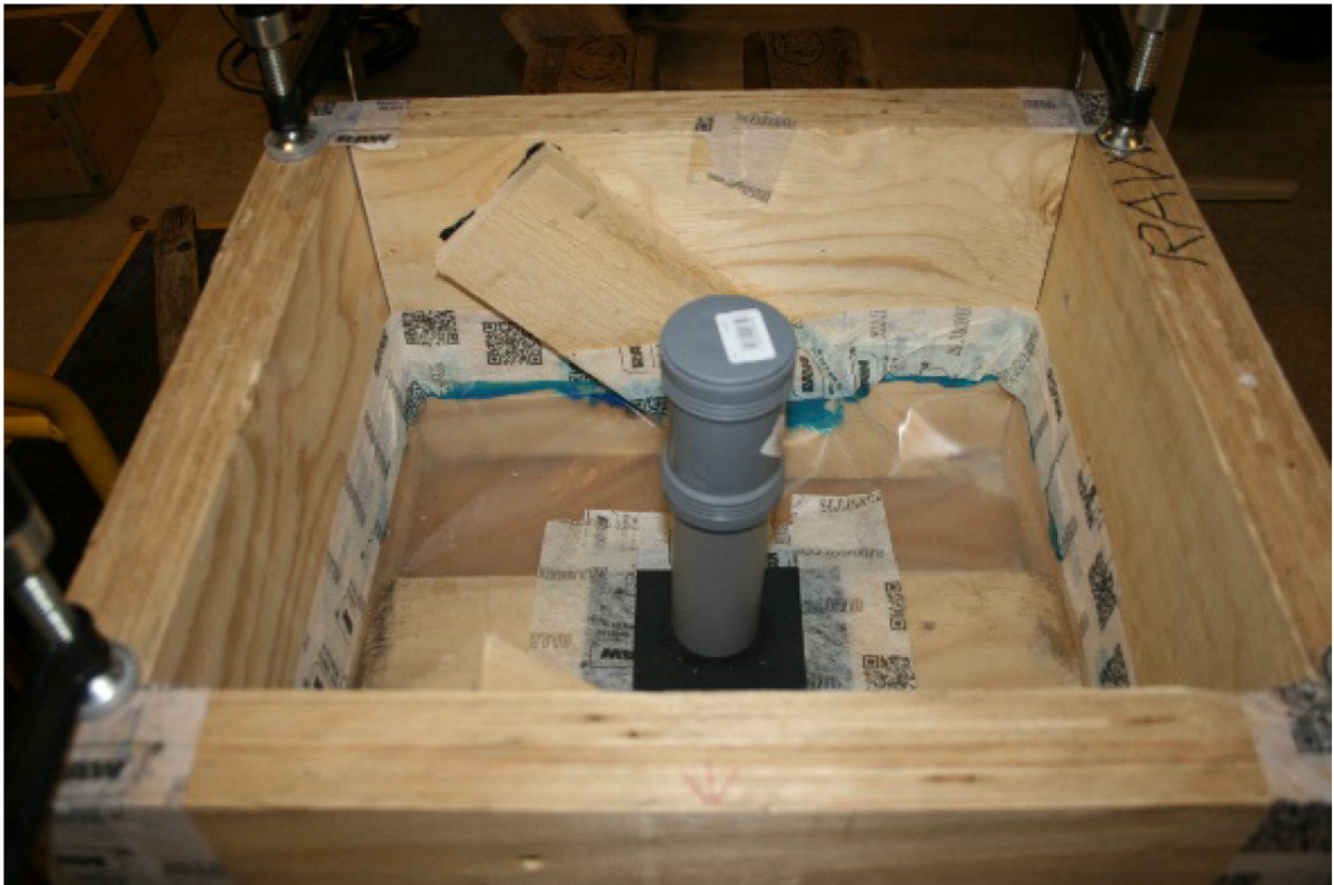
Figure 2.9: Test rig and sample simulating a roof section by Møller and Rasmussen (2020).
