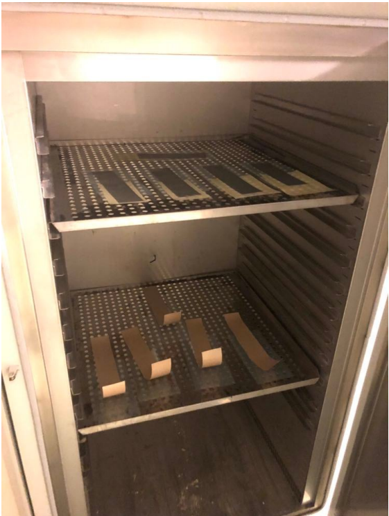
Figure 3.18: Peel resistance specimens in the heat chamber.
