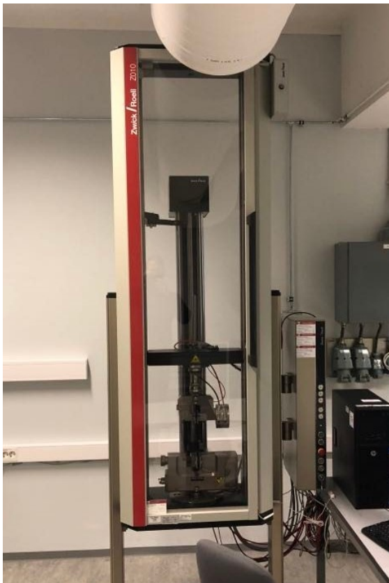
Figure 3.13: Zwick/Roell Z010 Material Tensile Testing Machine.
