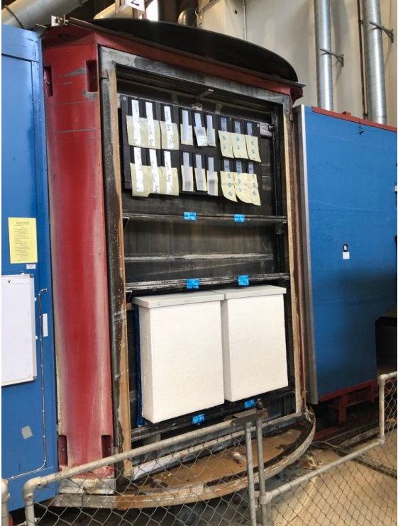
Figure 3.21: Peel resistance specimens in the upper half of the carousel.
