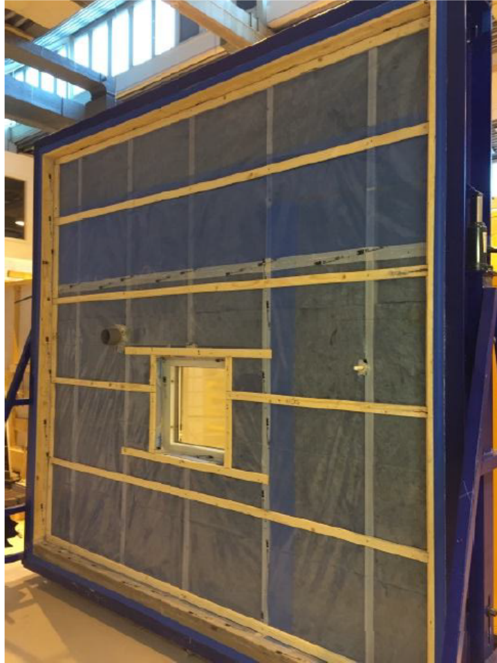
Figure 2.8: Full-scale wall assembly showing vapour barrier (Antonsson, 2017).
