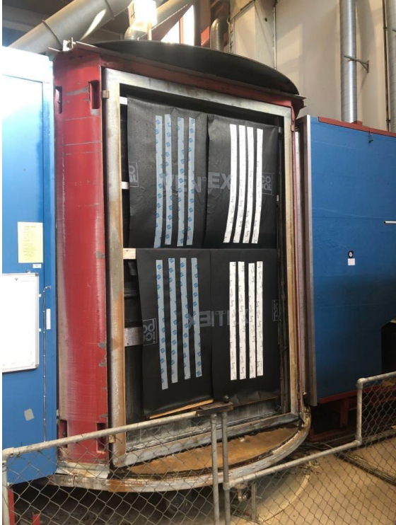
Figure 3.20: Air permeability specimens in the climate carousel.
