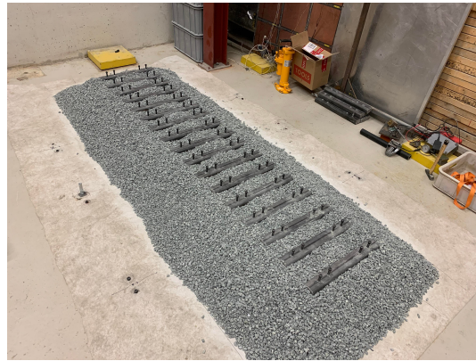
Figure 3.28.: Sleepers fully integrated into the ballast
