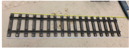
Figure 3.22.: Sleepers connected by rails
