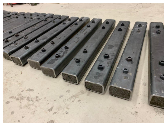
Figure 3.5.: Scaled sleepers filled with concrete
