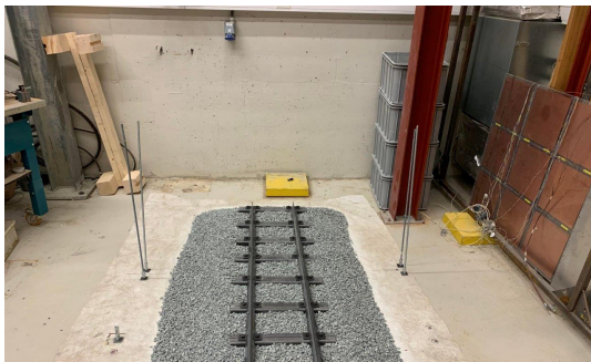
Figure 3.31.: Threaded rods fastened to the floor
