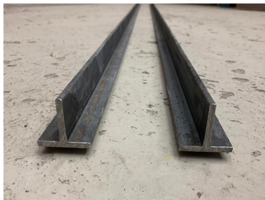
Figure 3.2.: Scaled rails' cross-section
