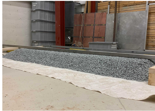
Figure 3.18.: Ensuring correct ballast height
