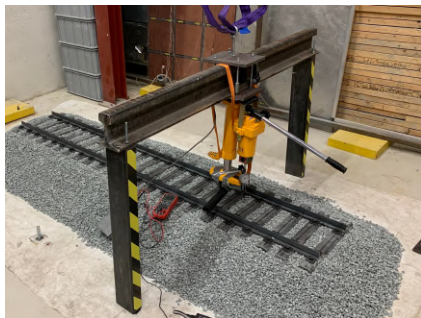
Figure 13: Vertical load test
