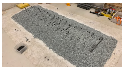
Figure 6: Integrating the sleepers Figure 7: Finalized scaled model
