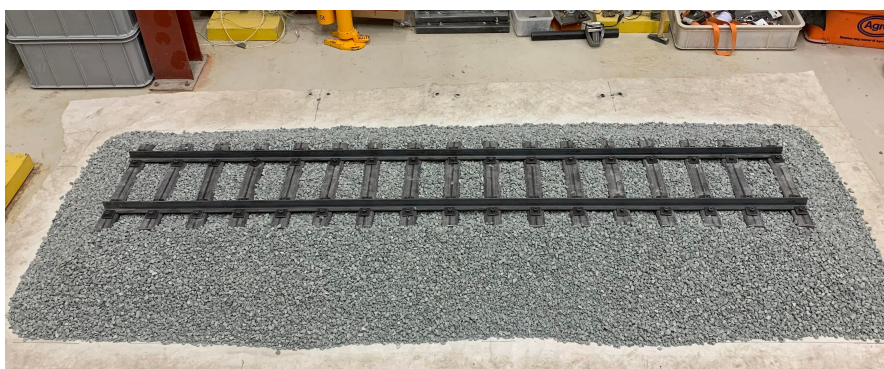
Figure 4.1.: The Wigaard track, a functional 1:5 scaled ballasted railway track
