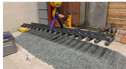
Figure 4: Sleepers connected by rails Figure 5: Structure lifted onto the ballast
