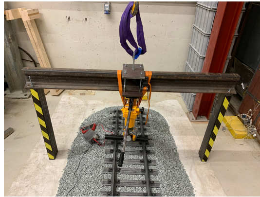
Figure 3.51.: Static vertical load set-up
