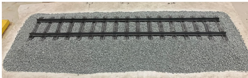
Figure 15: The Wigaard track, a 1:5 scaled ballasted railway track
