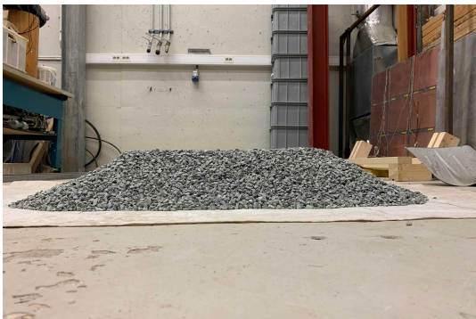
Figure 3.19.: Cross-section scaled ballast
