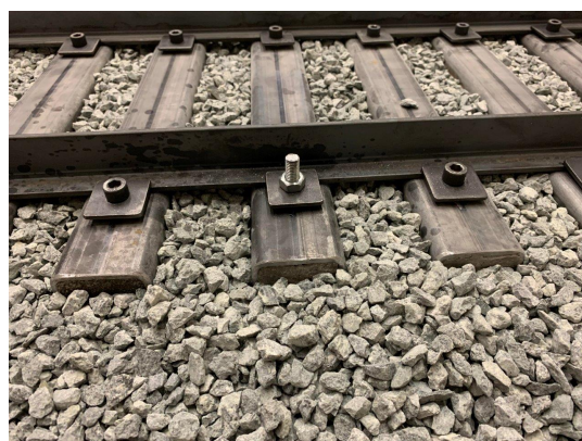
Figure 3.9.: Improved fastening solution for one damaged coupling nut
