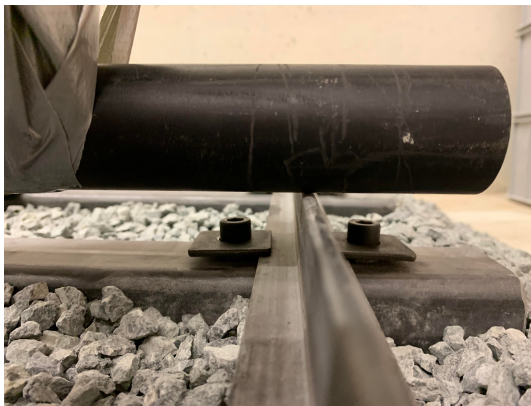
Figure 3.48.: Cylinder representing a wheelset
