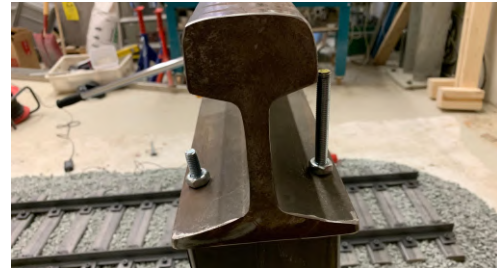
Figure 9: The rail as a beam, threaded rods, and fastening nuts
