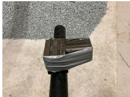
Figure 3.49.: Platform to measure vertical deflection
