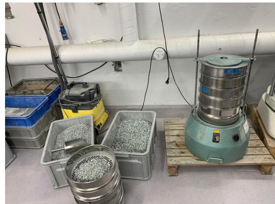
Figure 3.14.: Sieving machine and material
