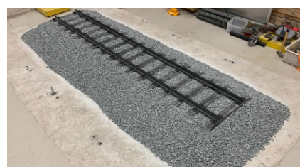
Figure 6: Integrating the sleepers Figure 7: Finalized scaled model
