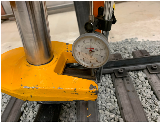
Figure 3.50.: Dial gauge placed on platform
