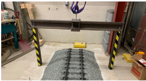
Figure 8: The frame spanning the scaled model
