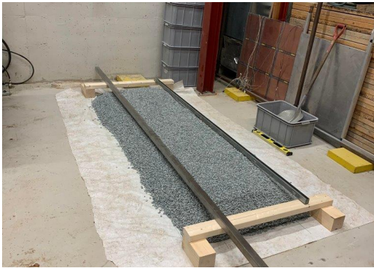
Figure 3.17.: Shaping the ballast layer
