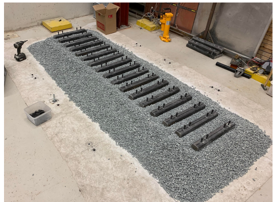
Figure 3.26.: Sleepers halfway integrated in the ballast
