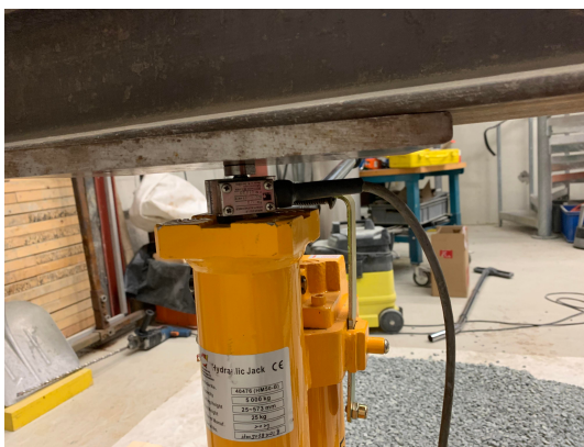
Figure 3.41.: Hydraulic jack in contact with load cell
