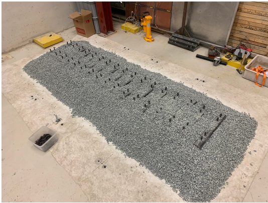
Figure 3.27.: Additional ballast material added
