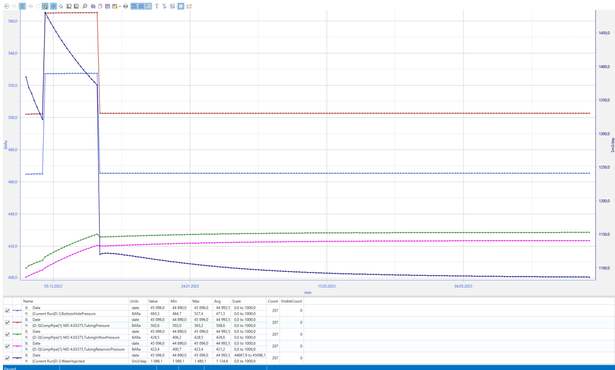
Figure 34: S5: Tubing pressures, reservoir pressure and water injection rate - initial injection temperature = 8 °C
