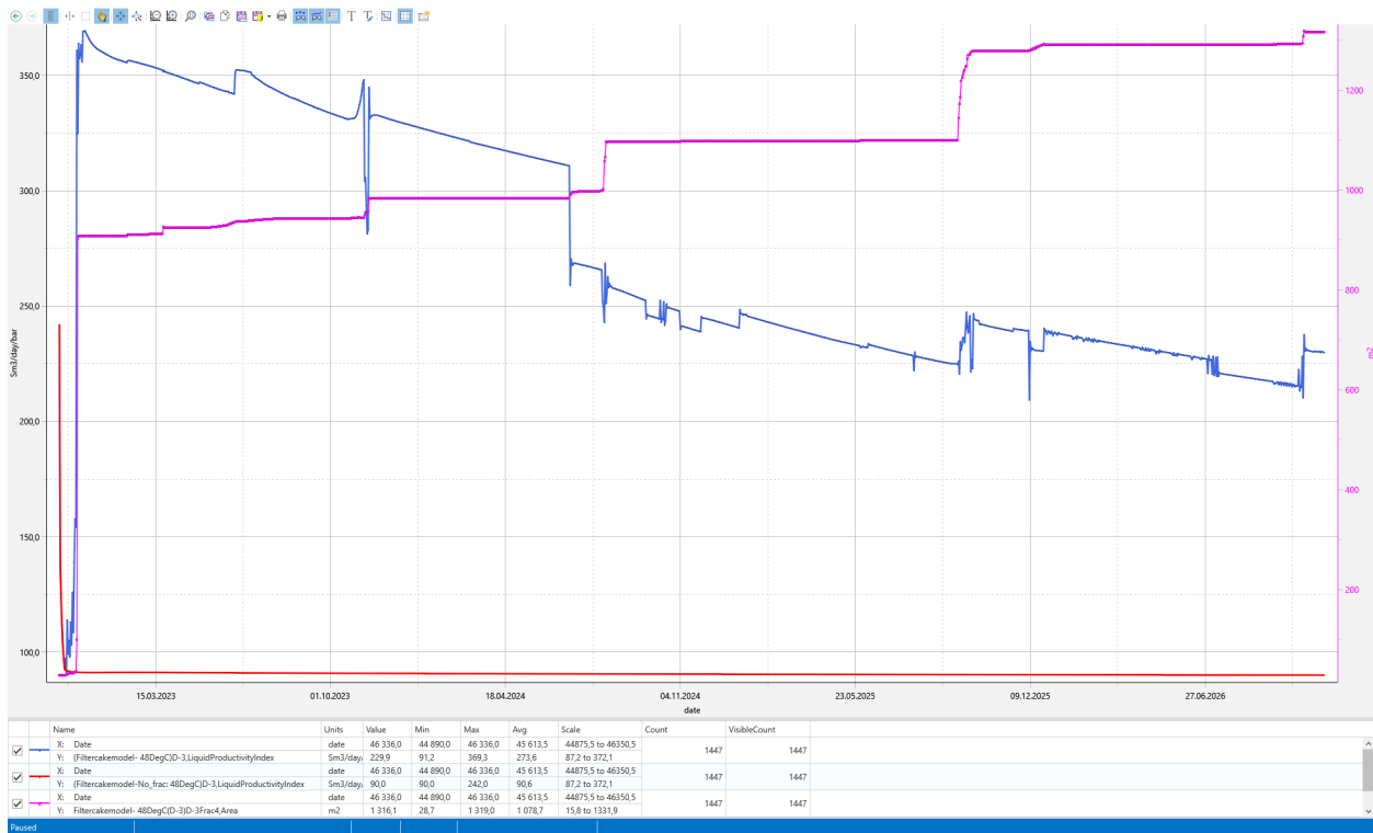
Figure 39: S8: Injectivity index for simulation run with filter-cake model - with/without fracture calculation, and fracture area (fracture seed 4)
