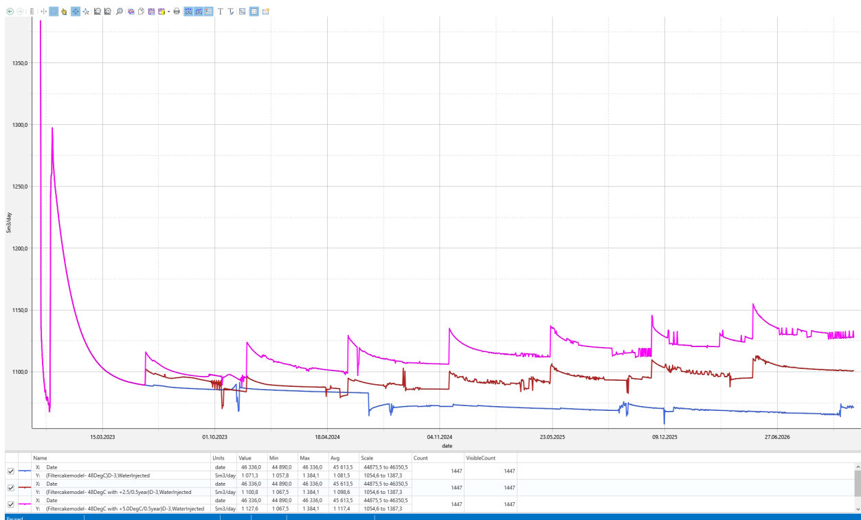
Figure 40: S8: Water injected [Sm³/day] for injection temperature of 48 °C, 48 + 2.5°C/0.5year, and 48 + 5 °C/0.5 year
