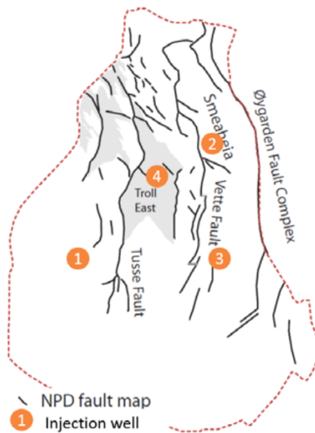
Figure 1.5: Potential storage site locations in the Horda CO 2 storage Hub. (1) Aurora structure, (2) Alpha structure, (3) Gamma structure, and (4) Troll Field (A. Lothe et al., 2019).
