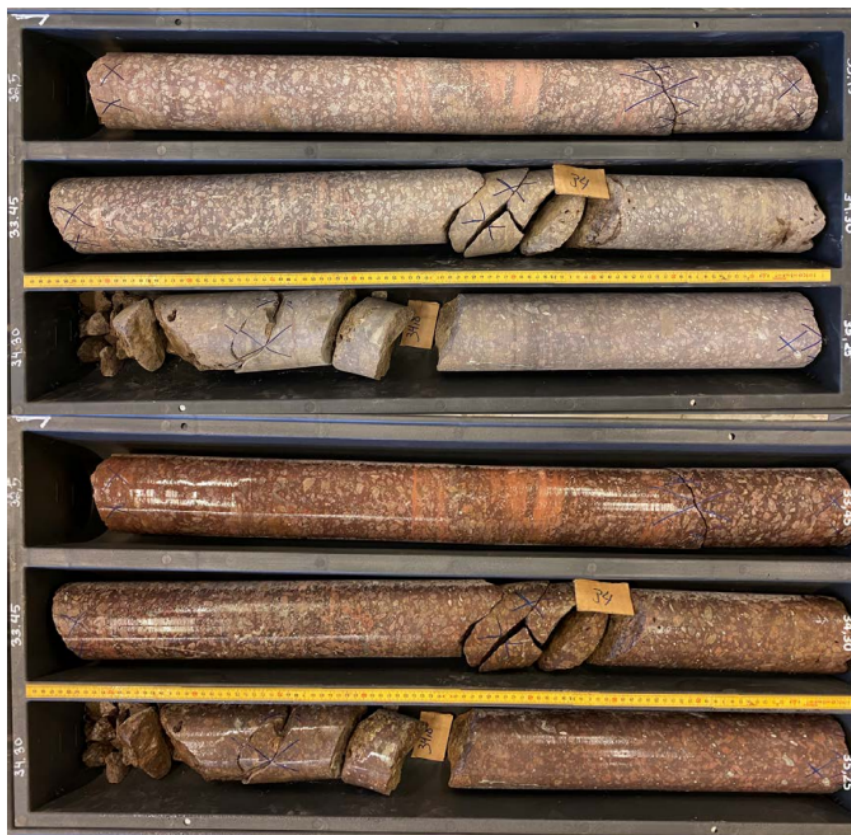
Figure 4.5: Core sample from "Rock_4", box 2, 32.5 – 35.25m, the rock core is dry at the top of the picture and wet at the bottom (NGI 2022).
