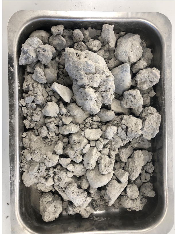
Figure 5.1: Material covered by grout removed from the sample.
