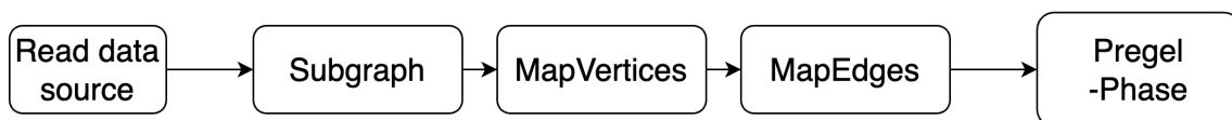
Figure 8.10: Shows the dataflow of operators used in preprocessing the graph before the pregel-phase.
