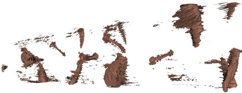
Figure 32: The knots segmentation of A1 timber board
