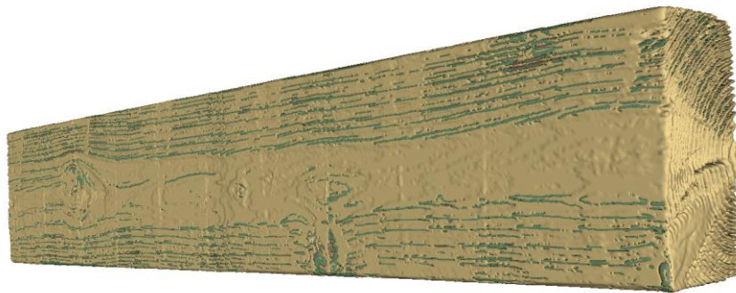
Figure 33: The combined segmentation of earlywood, latewood, and knots of A1 board
