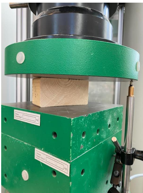
Figure 55: Lowside compressive testing
