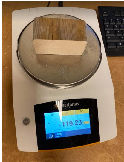
Figure 26: Weighing a sample from B1 board
