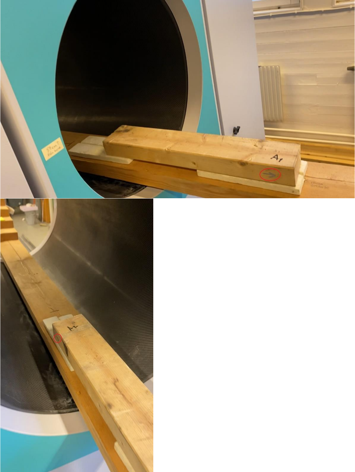
Figure 28: Preparing and placing the A1 and A2 board in the CT scanner
