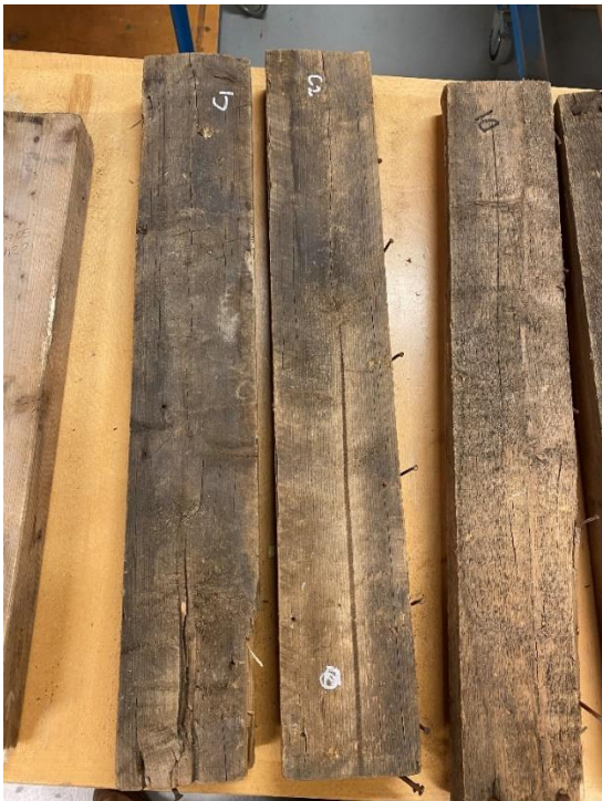
Figure 23: Preparing the timber boards for CT scanning
