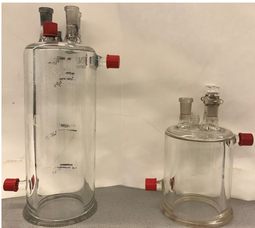
Figure 2.25: Example of two sonoreactors where the left one was increased only in height to facilitate larger scale sonochemical reactions. The diameter of the reactor remained unchanged.
