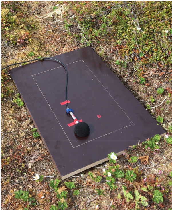
Figure 3. Flush-mounted microphone with windscreen on an ISO 1996–2-compatible ground plate.
