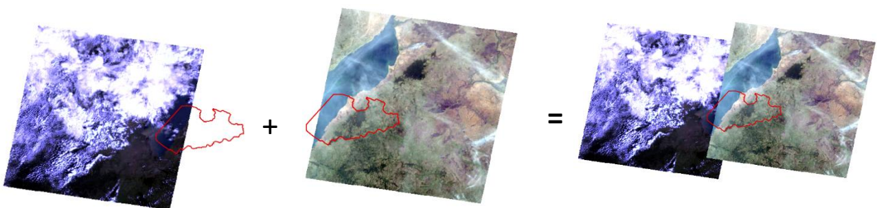
Figure 15: Mosaicking two dry season 1985 Landsat imagery from different scenes covering study area using the mosaic tool in ArcGIS Pro. (Author, 2023).
