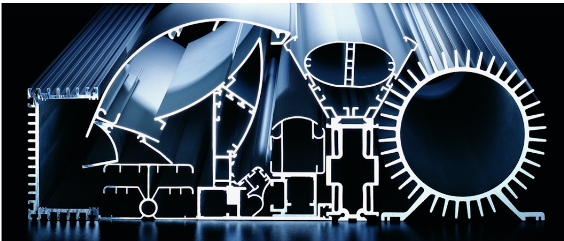
Figure 1.4.1: Some extruded profiles in aluminium ( Hydro extruded profiles 2022)
