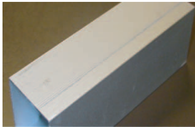
Figure 1.5.1: bearing washout lines in profile (Qamar, Arif, and Sheikh 2004)
