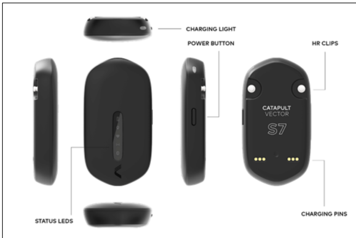
Figure 2.1: Catapult Vector S7. Notes: Tracking unit to collect GPS data during training and matches.
