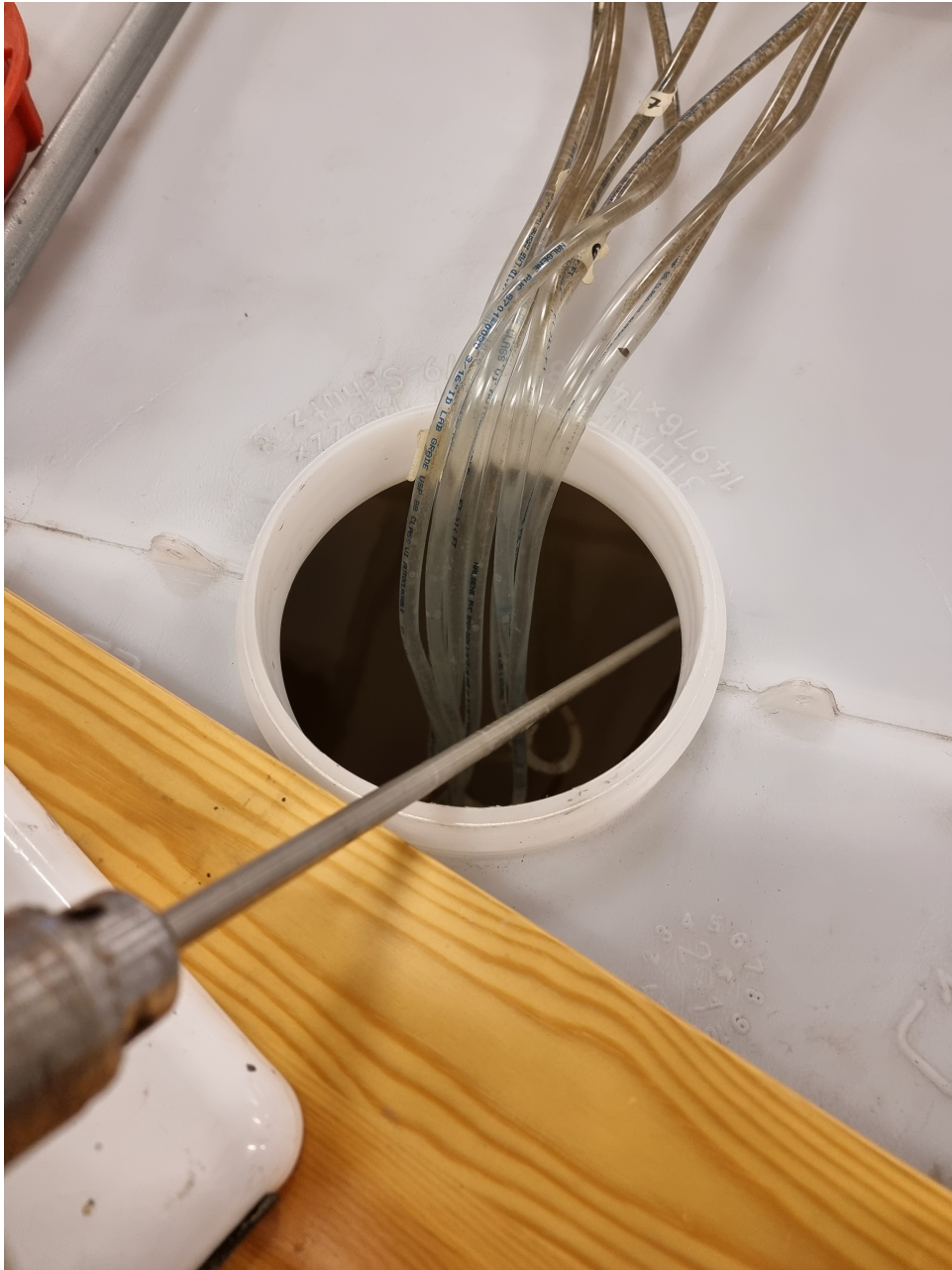
Figure 6.2: Water being transported from tank. A drill is there to avoid sedimentation.
