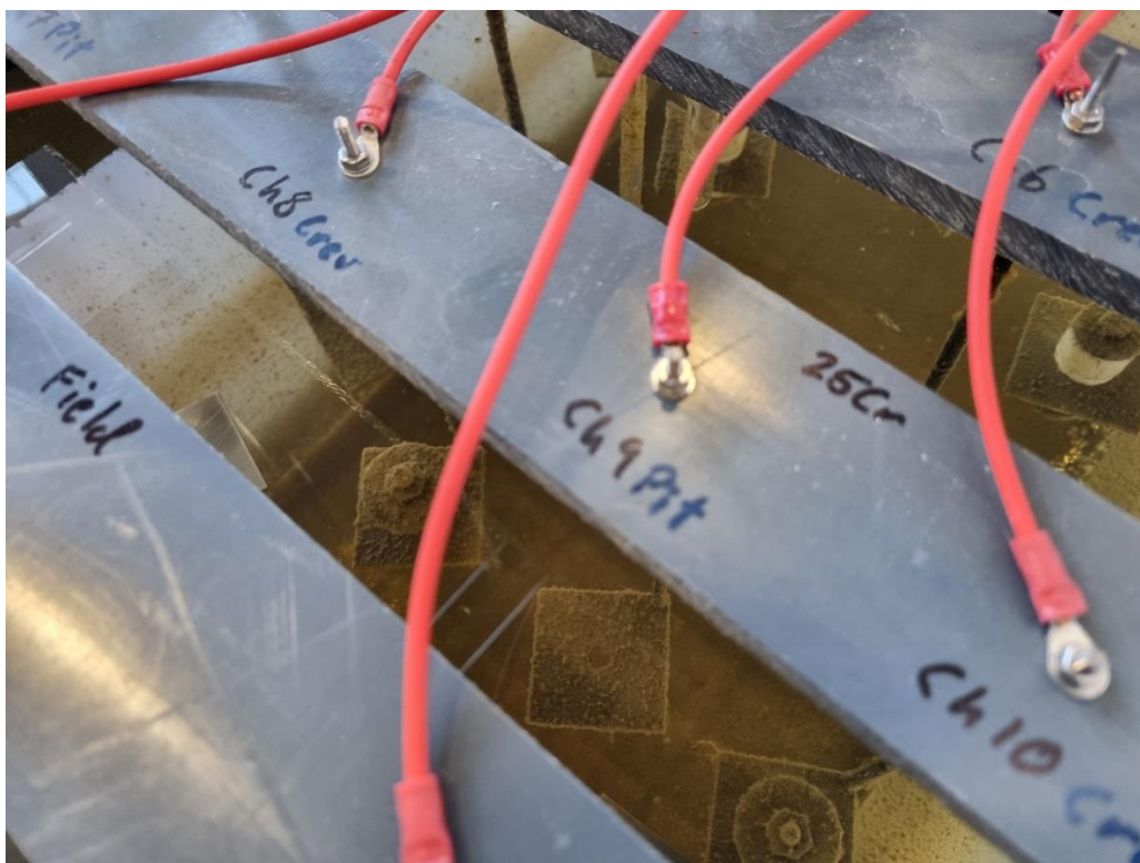
Figure 56: Particulates covering samples in on-site field experiment.
