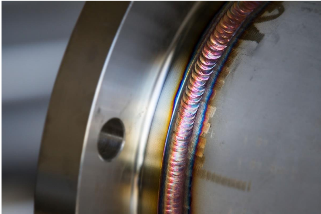
Figure 10: Weld scale. Note the color difference on the surface of the weld as well as the surrounding metal. Taken from https://www.bottlegases.co.uk/what-is-the-difference-between-tig-mig-welding/ on 04/06/2023.
