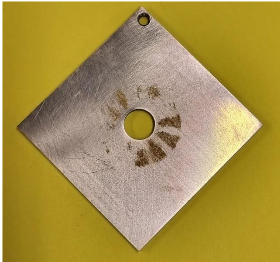
Figure 53: Corrosion attack on field-exposed sample of grade EN 1.4317.
