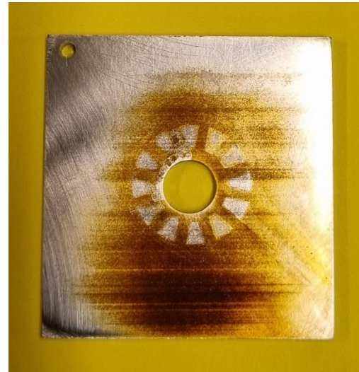
Figure 54: Corrosion attack on low-temperature laboratory experiment, grade EN 1.4317.
