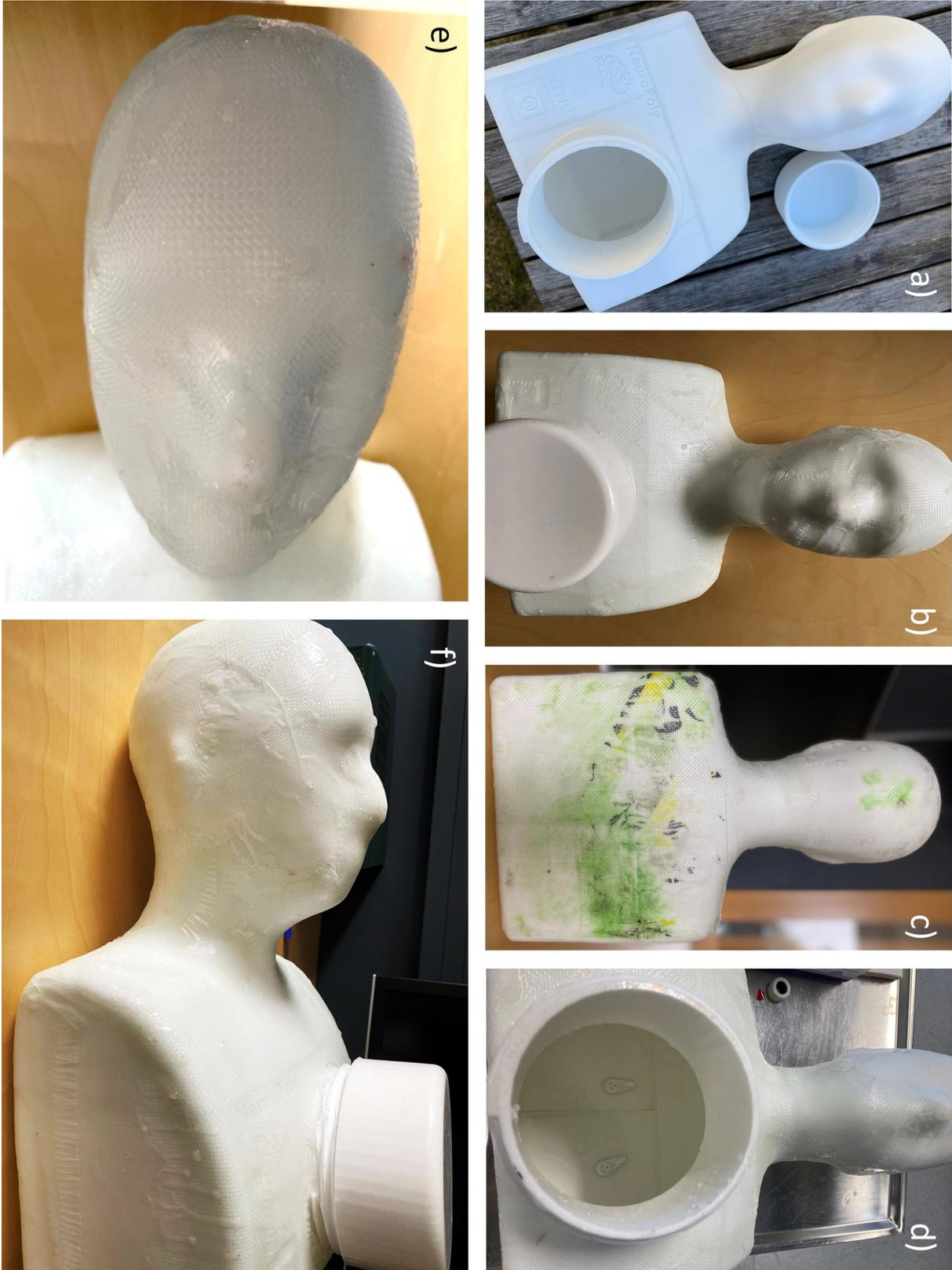
**Figure 4.18:** Pictures of the final shell of the phantom. It is presented before (a) and after (b,c,d,e,f) the epoxy and fiberglass application.
