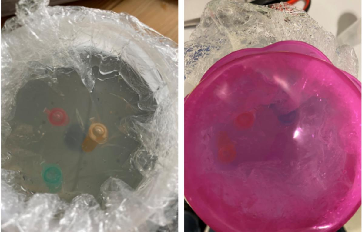
**Figure 3.3:** Set-up of the second experiment. The four tubes to be tested were inserted in a two-layer plastic film in the center of the plastic sphere, which was filled by a solution of salt, soap and distilled water.
