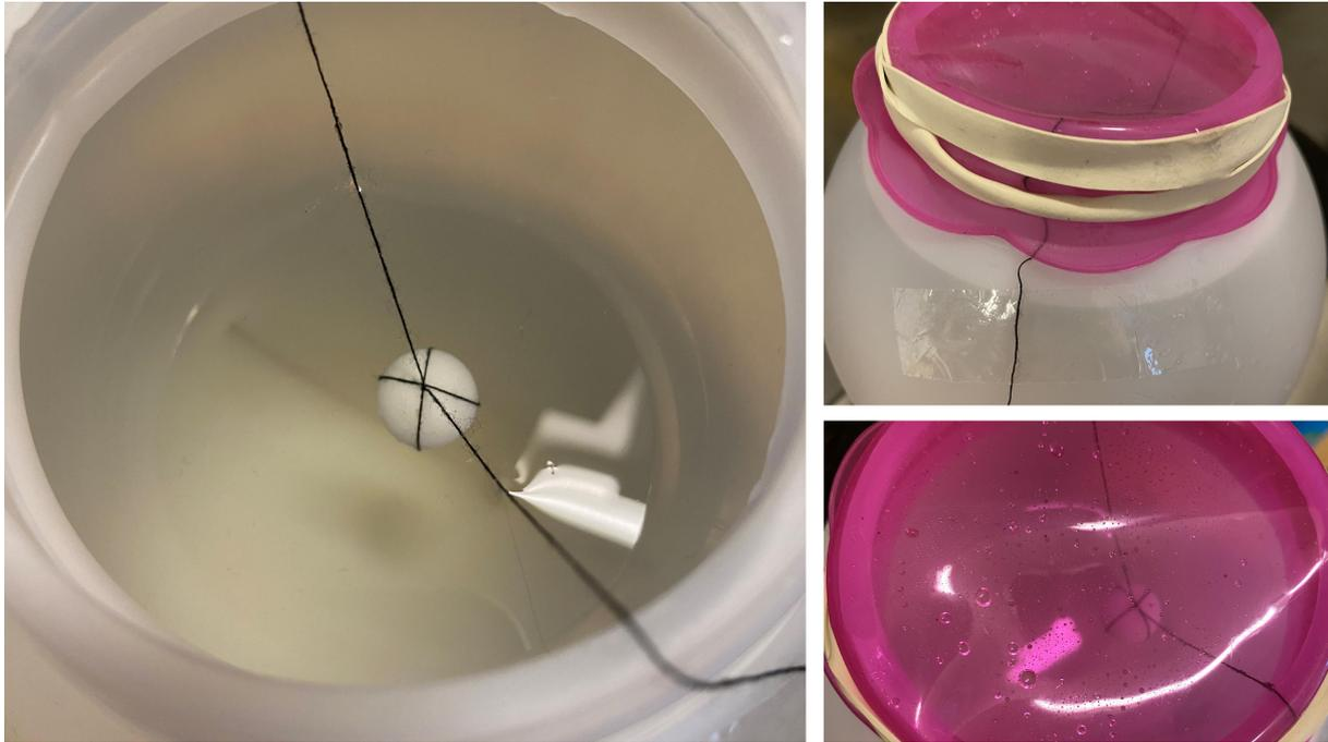
**Figure 3.1:** Set up of the first experiment: choice of the printing material. The sphere of the material to be tested is hung by two threads in the center of a plastic sphere filled with water, salt and soap. The assembly is closed by a reusable IKEA silicon lid and a rubber band to ensure water-tightness.
