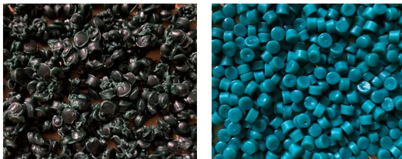
Figure 9. Low-grade recycled pellets on the left side and high-grade recycled pellets on the right side © Sidra Tul Muntaha 2022.
