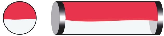
Fig. 22 Stratified flow of water and oil [SM]
