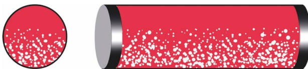
Fig. 20 Oil and dispersion of water in oil [O and Dw/o]
