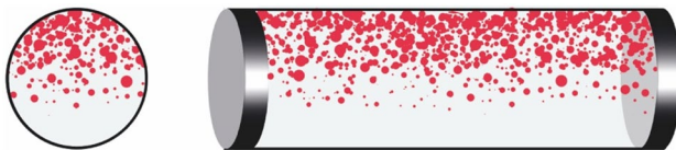
Fig. 19 Dispersion of oil in water and water [Do/w and W]
