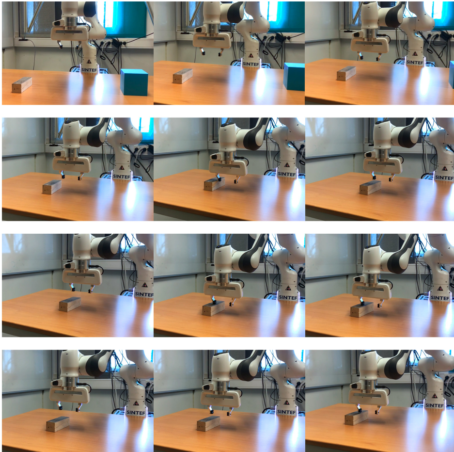
Figure 3.21: An example of a failed attempt. In this case, the robot loses height too quickly and ends up in a state next to the wooden block and never recovers. Even though it correctly goes back up, it misses again on both the second and third attempt at grasping, and ends up crashing into and pushing the block around.
