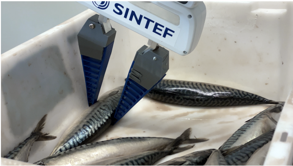
Figure 3.7: The robot performing a grasp predicted by the RAM. Often, as hypothesised in Sec. 3.1.2, after a few picks, the remaining fish in a box are lying along the walls. In these cases, the trained model consistently displays good obstacle avoidance, slightly touching the side and the bottom, as it has to, in order to grasp successfully.
