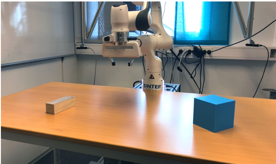
Figure 3.16: The test setup for the experiment conducted in this section. The goal for the robot is to pick up the small wooden block and place it on the larger blue cube.
