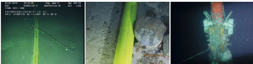
FIGURE 2.12. Example of external debris - misplaced objects 25 © Anonymous Operator
