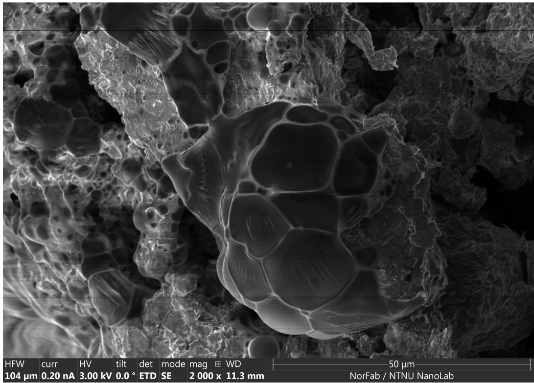
Figure C.4: SEM image of a bubble on the anode surface of a cell cycled at 5°C at 65% SoH
