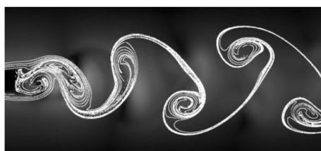
Figure 2.42: Visualization of a Karman vortex street forming at the trailing edge of a blade and moving downstream [26].
