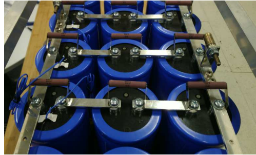
Fig. 6: Photos of the laboratory prototypes of SIRIUS converter and the two different capacitor banks
