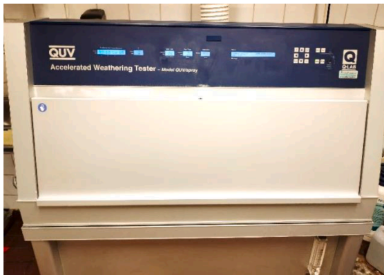
Fig. 2. Accelerated weathering tester (Model QUV/Spray).
