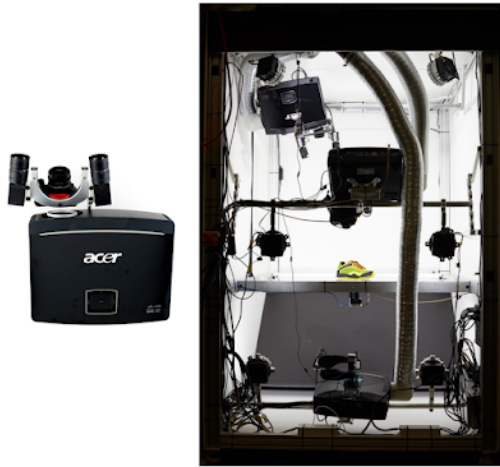
Figure 3.1.1: Setup of Google’s scanning rig for high-quality model creation [49]
