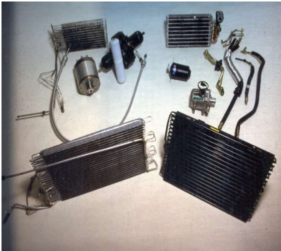
Figure 1A: CO 2 prototype system (left) and BMW 520 R-12 system (right). 1B: Coefficient of Performance (COP) as a function of ambient air temperature for various operating conditions.
