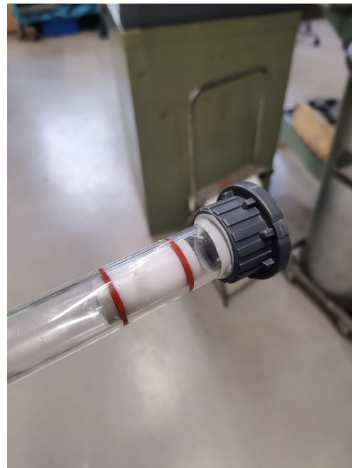
Figure 7.4: Closeup of new glass tube with new piston and o-rings
