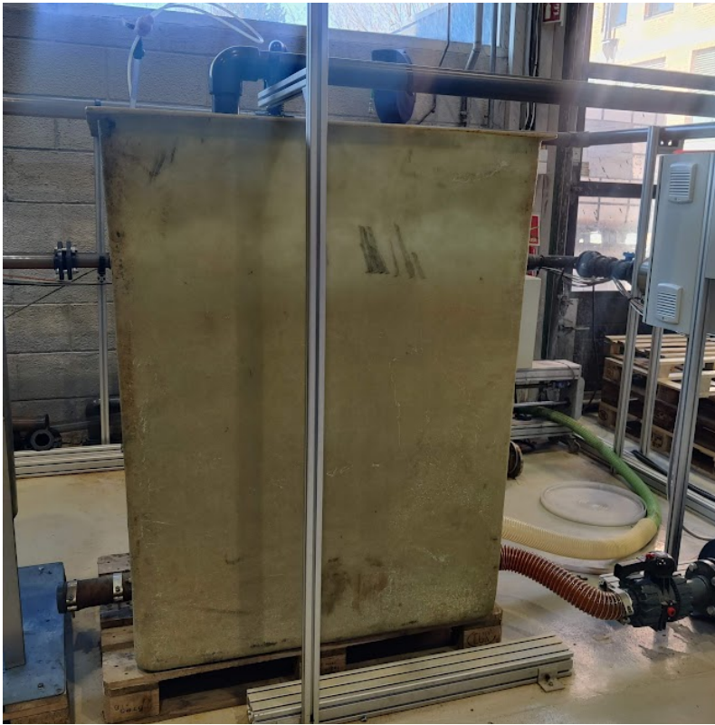
Figure 4.3: Sand separation system
