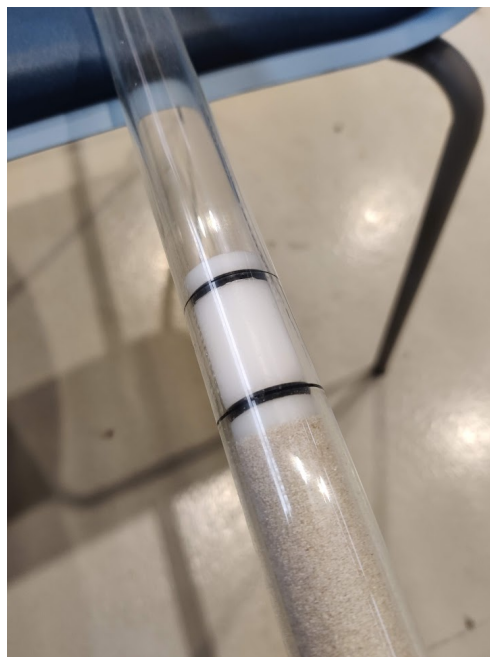
Figure 7.2: Closeup of old glass tube with piston and o-rings
