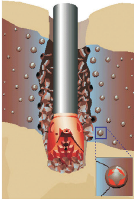
Figure 29: Drilling through induced over-pressured shale
