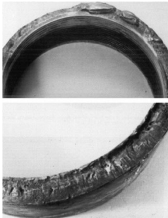
Figure 22: Post-separation damage to fracture surfaces of a BHA connection. (Macdonald 2007)
