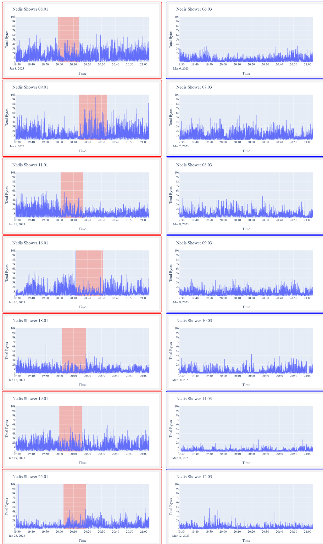
Figure 5.42: Graphs of traffic flows from the showering events measured in bytes with event graphs framed in red and baseline graphs framed in blue for Nedis. Event times are marked in red on the event graphs.
