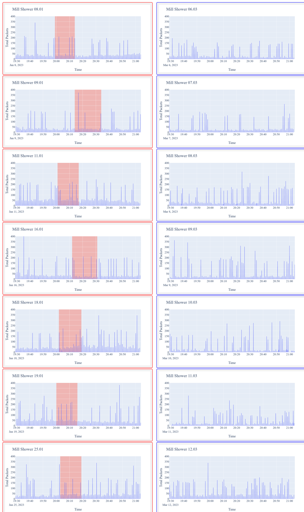
Figure 5.34: Graphs of traffic flows from the showering events measured in packets with event graphs framed in red and baseline graphs framed in blue for Mill. Event times are marked in red on the event graphs.
