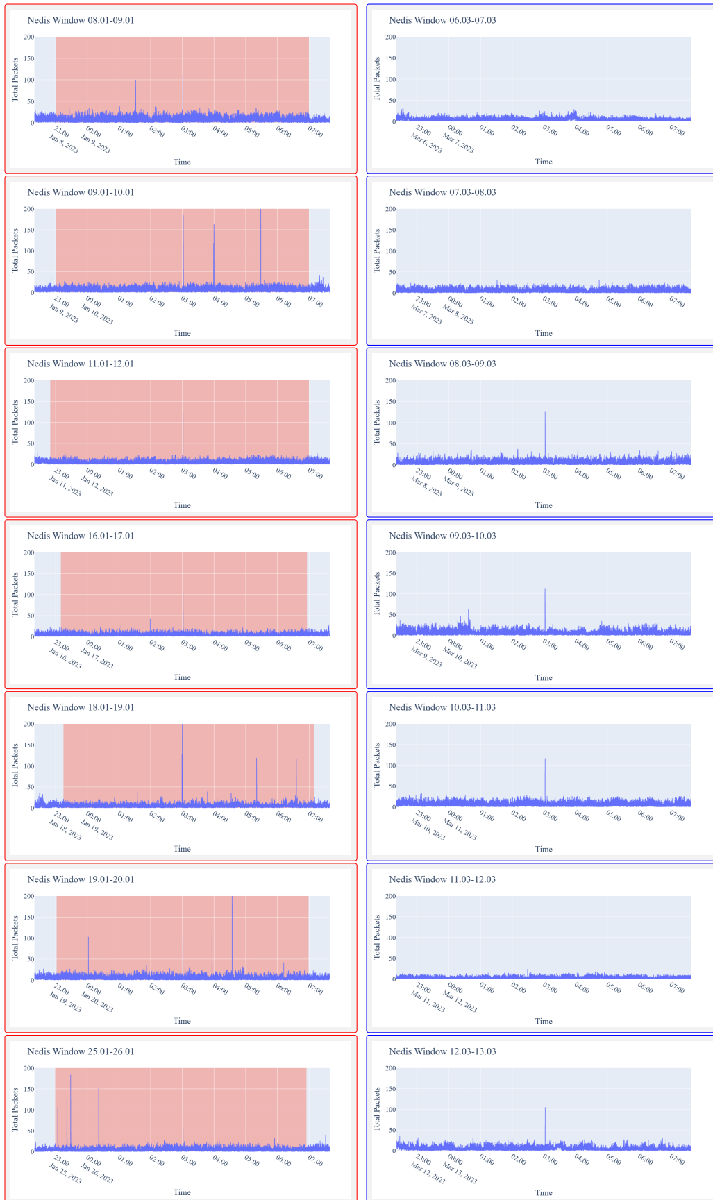
Figure 5.54: Graphs of traffic flows from the window open events measured in packets with event graphs framed in red and baseline graphs framed in blue for Nedis. Event times are marked in red on the event graphs.
