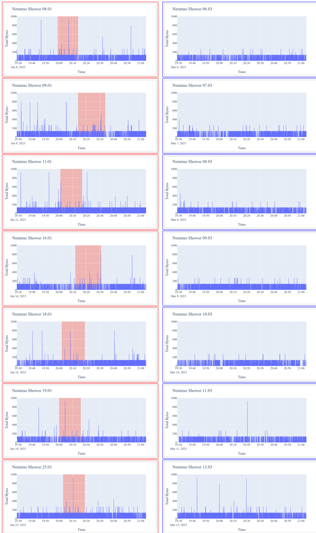
Figure 5.32: Graphs of traffic flows from the showering events measured in bytes with event graphs framed in red and baseline graphs framed in blue for Netatmo. Event times are marked in red on the event graphs.
