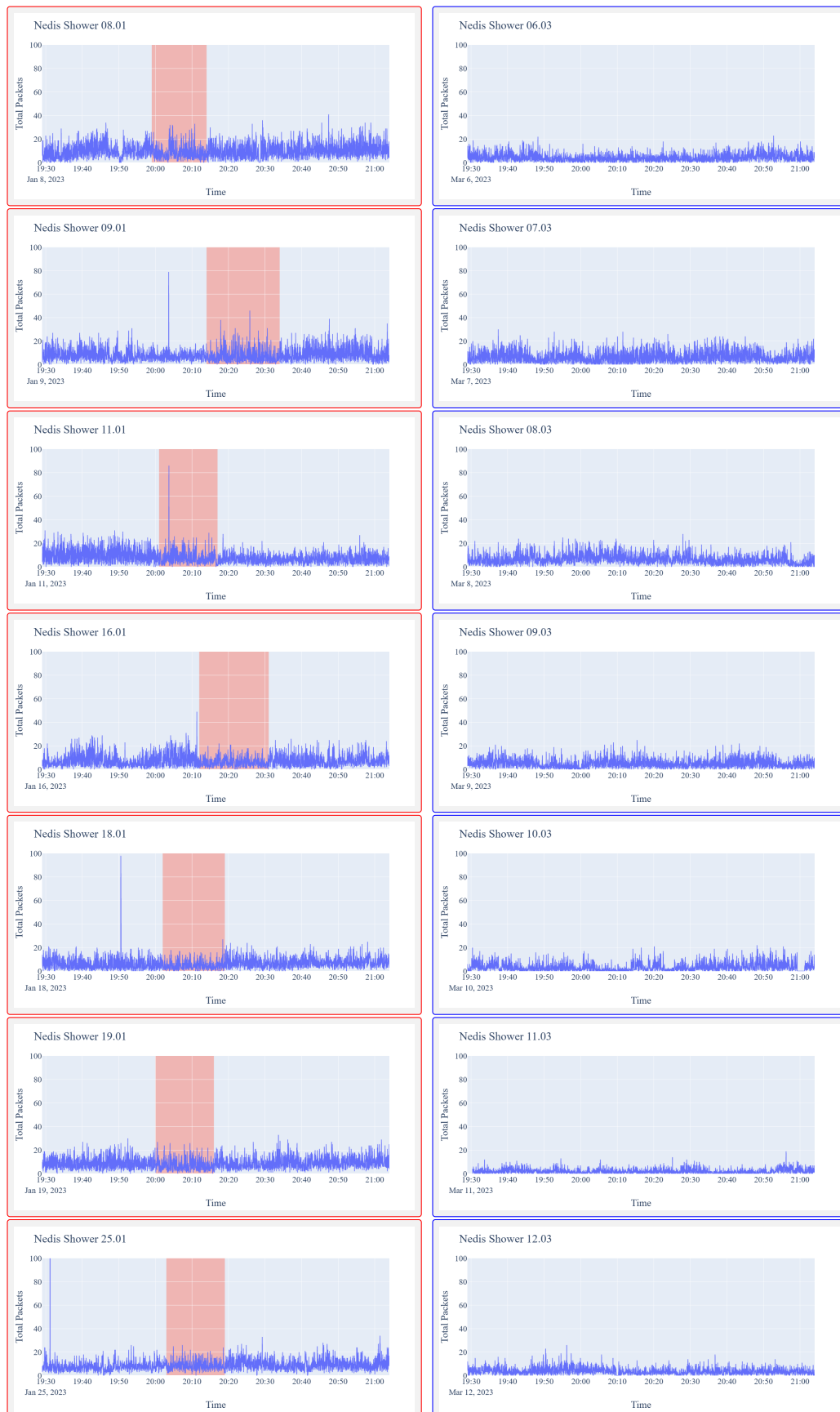
Figure 5.39: Graphs of traffic flows from the showering events measured in packets with event graphs framed in red and baseline graphs framed in blue for Nedis. Event times are marked in red on the event graphs.
