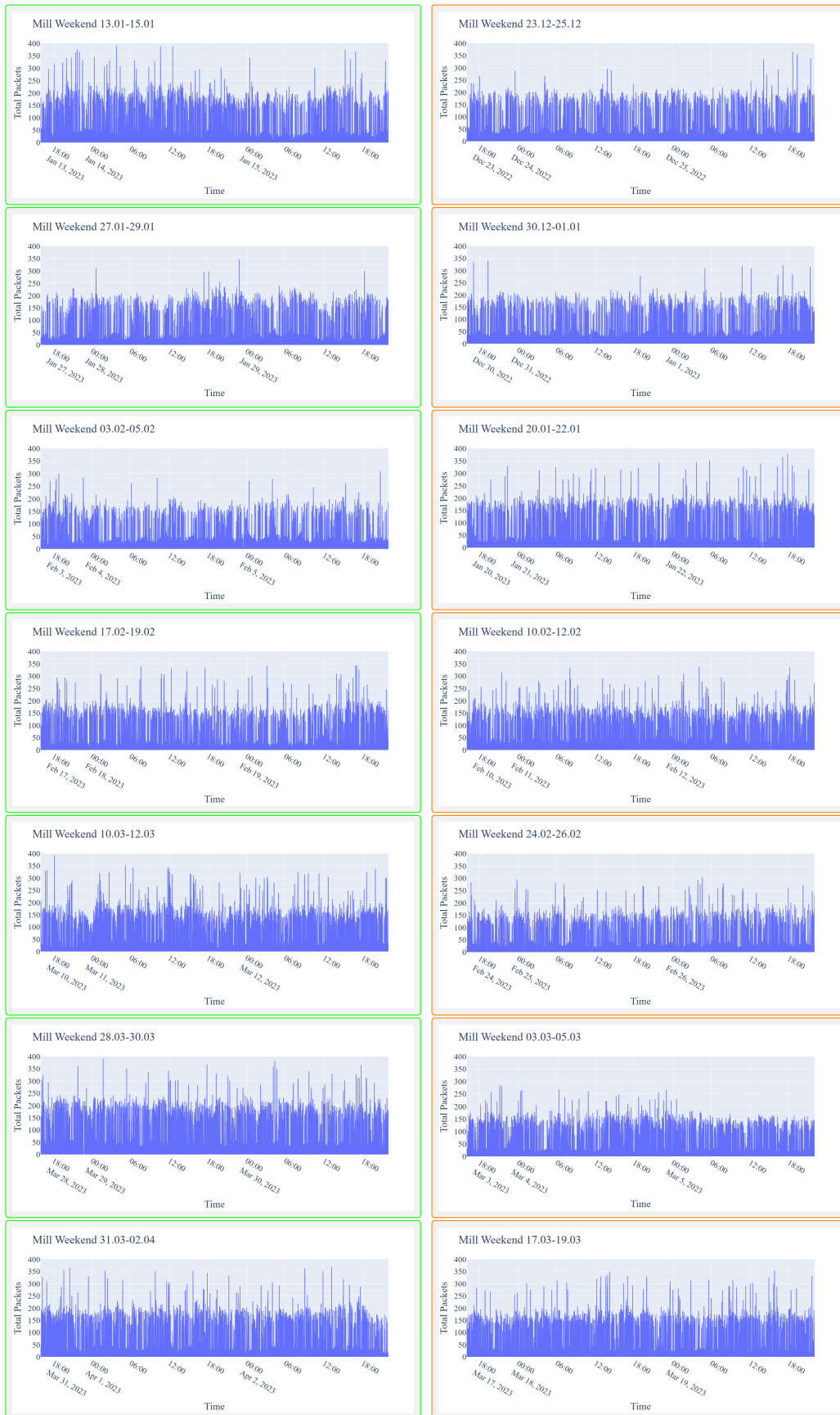
Figure 5.63: Traffic patterns for weekends at home, marked in green, and gone, marked in orange, measured in total amount of packets sent and received for Mill during the weekends
