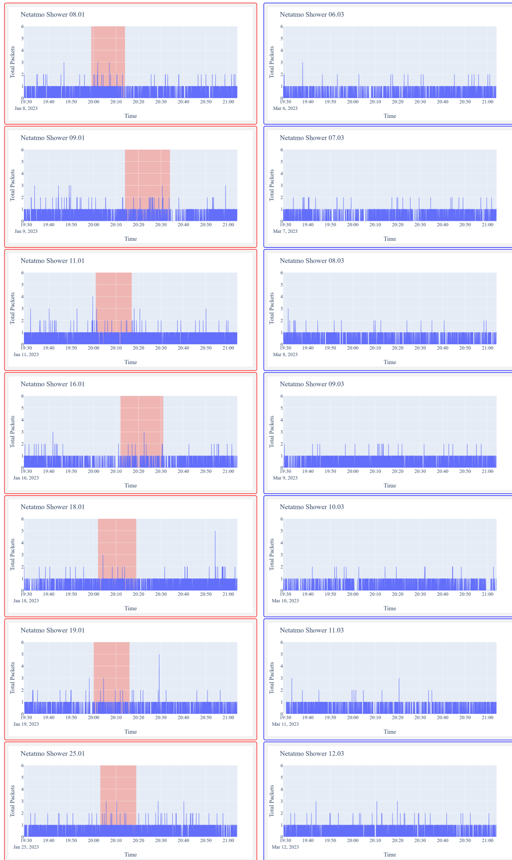
Figure 5.29: Graphs of traffic flows from the showering events measured in packets with event graphs framed in red and baseline graphs framed in blue for Netatmo. Event times are marked in red on the event graphs.
