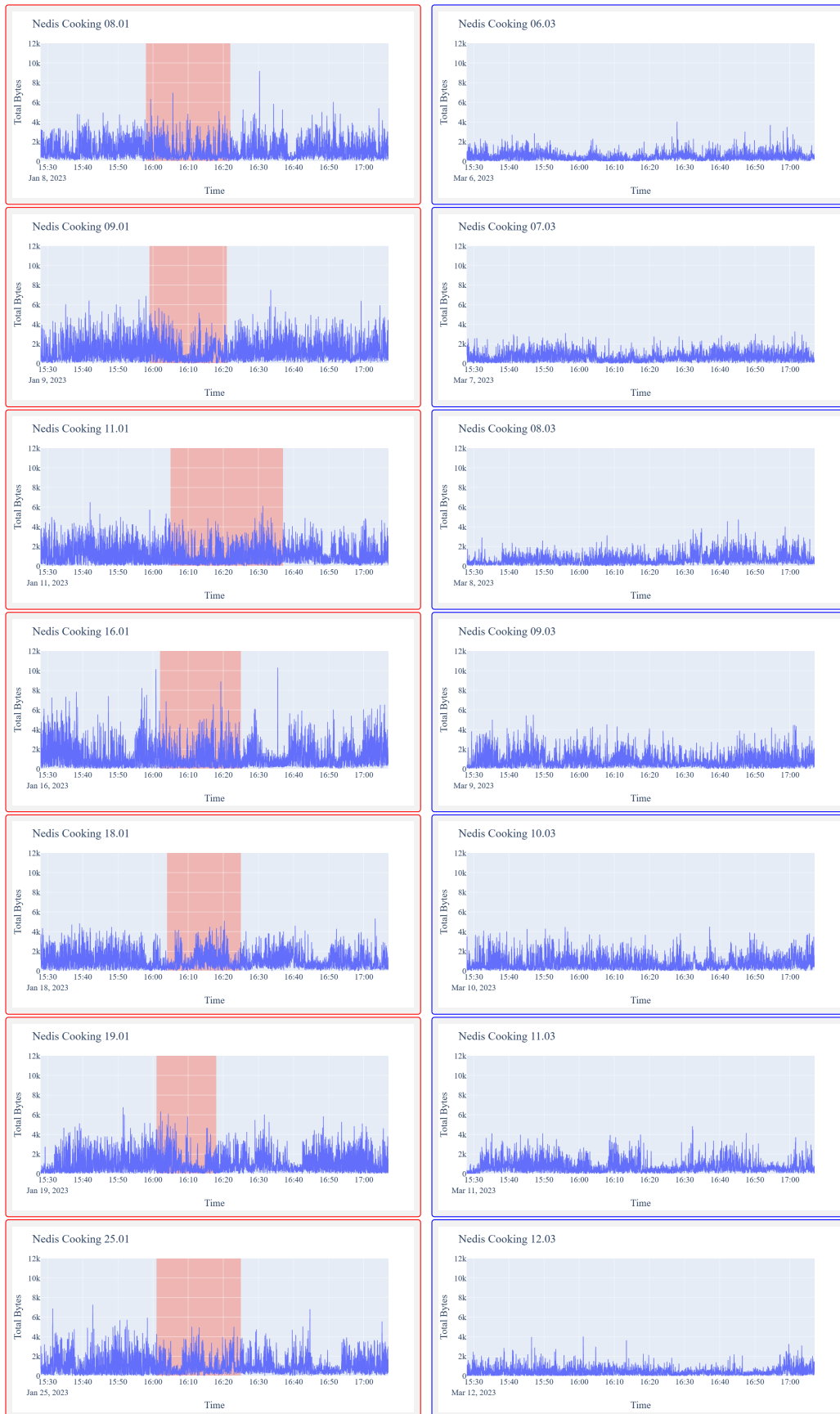
Figure 5.27: Graphs of traffic flows from the cooking events measured in bytes with event graphs framed in red and baseline graphs framed in blue for Nedis. Event times are marked in red on the event graphs.
