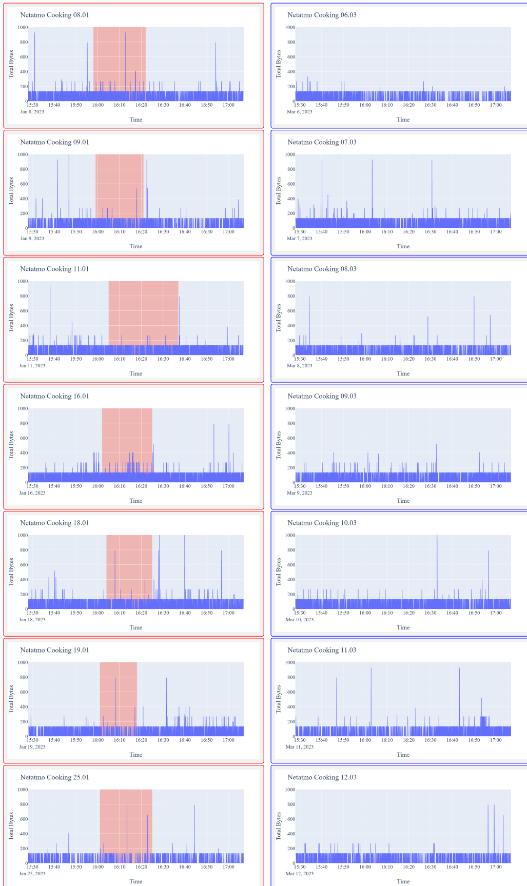
Figure 5.17: Graphs of traffic flows from the cooking events measured in bytes with event graphs framed in red and baseline graphs framed in blue for Netatmo. Event times are marked in red on the event graphs.
