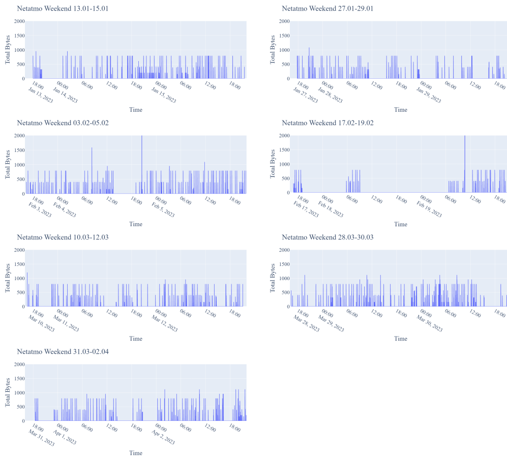
Figure 5.60: Traffic patterns for weekends at home with filtered with packets over 154 bytes for Netatmo
