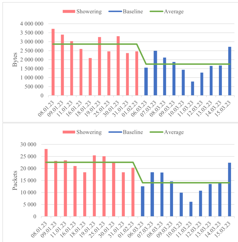
Figure 5.38: Graphical presentation of event and baseline shower calculations with packets and bytes, including average value extracted from Table 5.24 for Nedis
