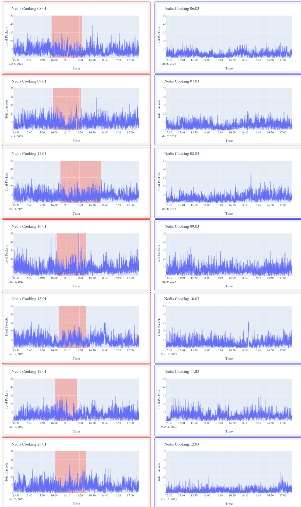
Figure 5.24: Graphs of traffic flows from the cooking events measured in packets with event graphs framed in red and baseline graphs framed in blue for Nedis. Event times are marked in red on the event graphs.
